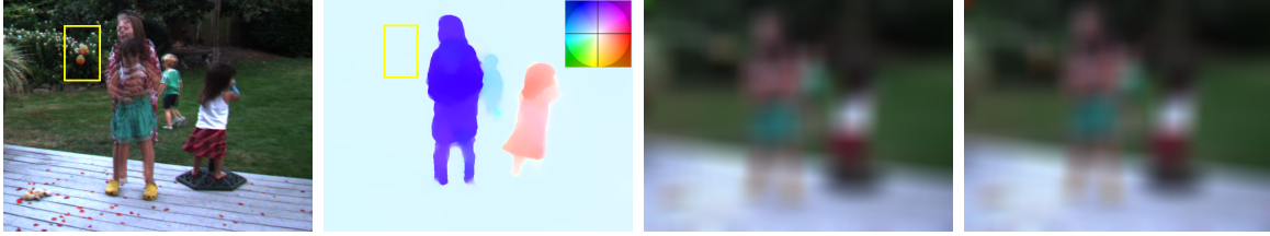
Figure 2.1: Small things moving fast. 1st: two images from the Middlebury dataset (shown superimposed) with the fast-moving ball highlighted, a classic failure mode of multi-resolution optical flow (2nd: the inset color wheel shows the map from color to image displacement). Small objects disappear at coarse resolution, where large motions are computed (3rd, 4th), and are never recovered in a differential-based variational scheme.
