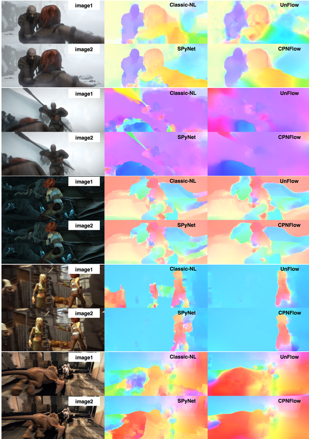
Figure 3.5: Visual comparison on MPI-Sintel. Variational: CClassic-NL [SRB10], Supervised: SPyNet [RB17], Unsupervised: UnFlowC [MHR18] and our CPNFlow-C.
