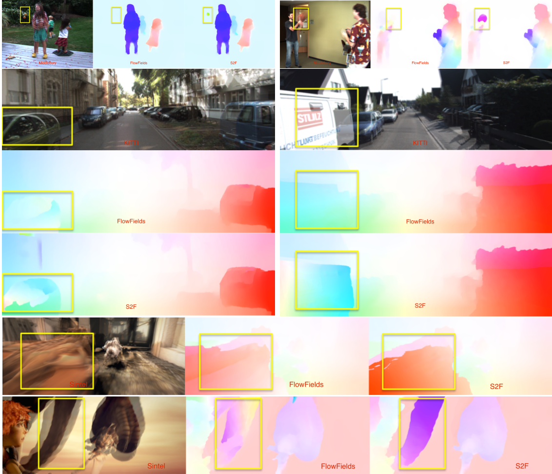
Figure 2.4: Representative samples from various datasets: Middlebury (row 1), KITTI (rows 2, 3, 4), Sintel (rows 5,6). We compare the component flow [BTS15] (FlowFields), with ours (S2F). Details are highlighted in yellow rectangles.
