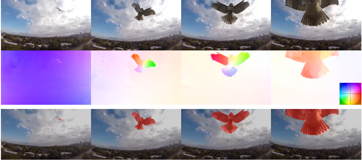
Figure 6.1: An encounter between a hawk and a drone (top). The latter will not survive without being aware of the attack. Detecting moving objects is crucial to survival of animal and artificial systems alike. Note that the optical flow (middle row) is quite diverse within the region where the hawk projects: It changes both in space and time. Grouping this into a moving object (bottom row) is our goal in this work. Note the object is detected by our algorithm across multiple scales, partial occlusions from the viewpoint, and complex boundaries.
