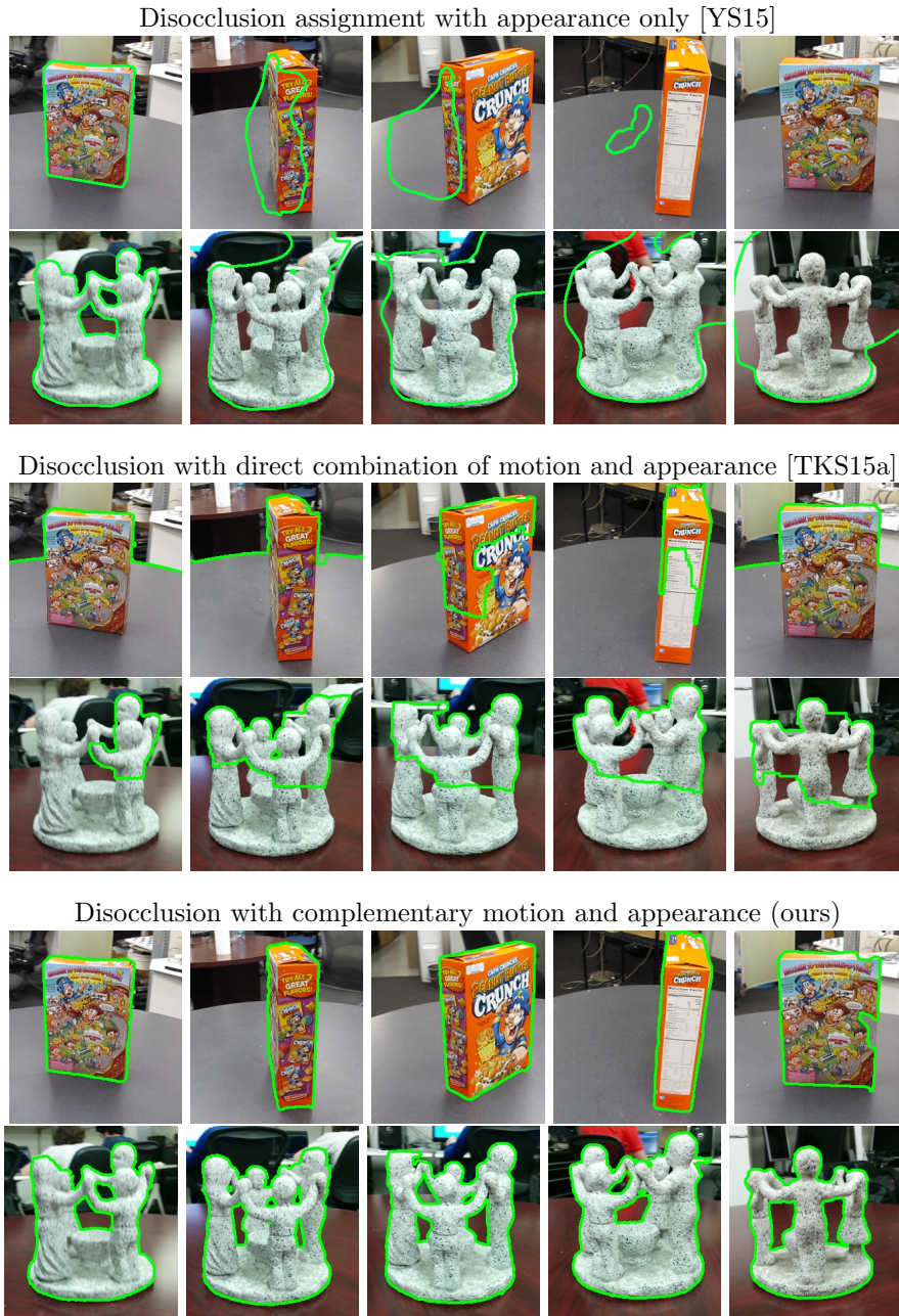
Figure 5.3: Rotating around an object. Disoccluded parts of an object that have different appearance than the visible parts in the previous frame (cereal box) pose difficulties to existing algorithms. Labeled above are various strategies for addressing disocclusions. To show that our method performs even under self-similar appearance, we have included the statue.
