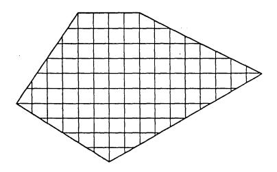
Figure 5. Comparison of the computational grid created by the program FMMG and a rectangular grid, for the problem of liquid absorption into a polygonal block.
