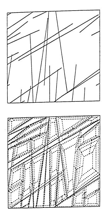
Figure 4. (a) Two-dimensional flow region containing a network of fractures; (b) Discretization of flow region in integrated-finite-difference format, using FMMG.
