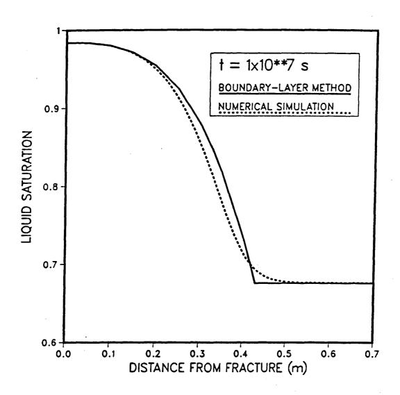
Figure 1. Saturation profiles for one-dimensional absorption in Topopah Spring welded tuff. Physical properties of tuff are listed in text.
