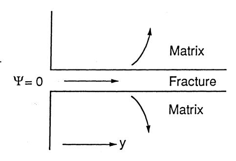
Figure 2. Schematic diagram of the problem of infiltration into a fracture, with transverse leakage into the matrix.
