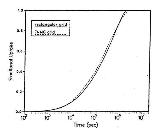
Figure 6. Fractional uptake of liquid for the problem shown in Fig. 4, calculated with TOUGH, using an FMMG grid and a rectangular grid.
