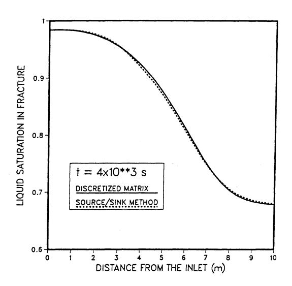
Figure 3. Saturation profile in fracture for flow along fracture with transverse leakage to matrix. Hydraulic properties used in simulations are listed in text.
