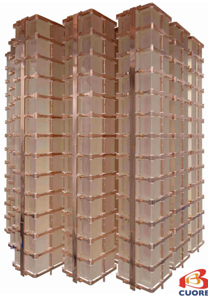
Fig. 1. The complete CUORE detector: The 19 towers hosting the 988 \text{TeO}_2 crystals.
