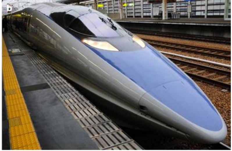
Figure 1.4 (a) The kingfisher bird dives into water without creating a splash due to its beak shape[9]. (b) The Shinkansen nose cone design was inspired by the kingfisher beak [10].
