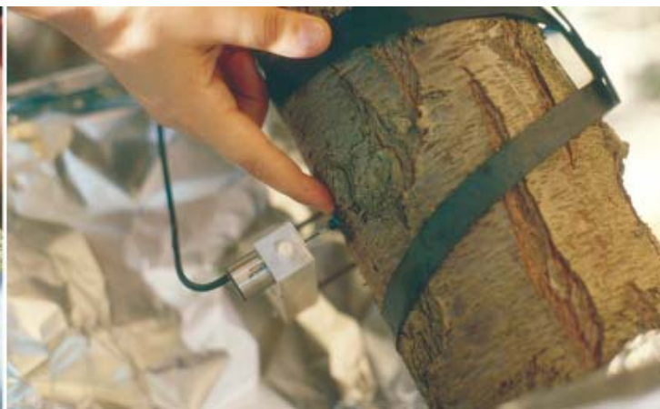
Linear variable differential transformers (LVDTs) continuously recorded the diameter of primary tree scaffolds. Maximum daily trunk shrinkage (MDS) data was used as a water-stress indicator to schedule regulated deficit irrigation (RDI).
