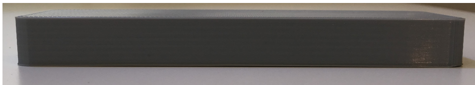
Figure 5.8: Flat rectangular prism with fillets printed on the LulzBot printer, showing a small amount of warpage, with center of part deformed so that it is higher than the sides.
