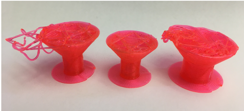
Figure 5.11: Three attempts to print versions of the tapered cylinder part that became dislodged from printer platform, causing the print to fail.
