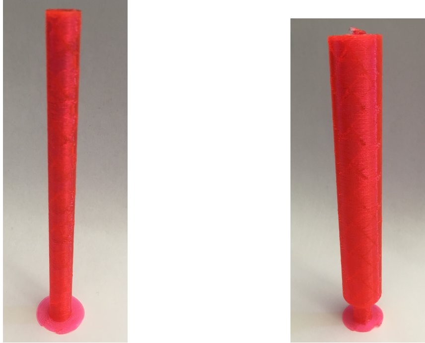
(i) Cylinder part (130 mm \times 10 mm) (ii) Tapered cylinder part (140 mm \times 10-20 mm)
