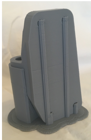
Figure 5.20: GE bracket printed at Orientation 2. Support material is visible under the holes and on the backside of the part, supporting the angled features.
