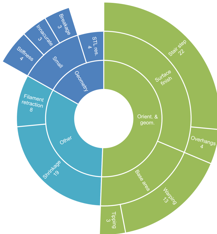
Figure 3.2: Students described a variety of issues relating to orientation, geometry, and printer settings. The reported issues are grouped into categories, and the number of students reporting each issue is listed.
