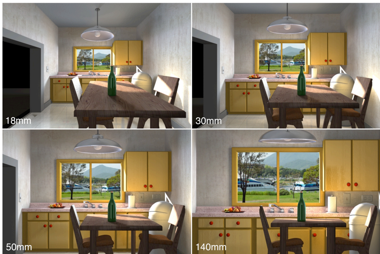
Figure 3.2. Frames from a dolly-zoom shot of a kitchen. Using Maya (Autodesk), we imaged a 3D model of a kitchen (Birn, 2008) while simultaneously zooming in and dollying out. The angle subtended by the
