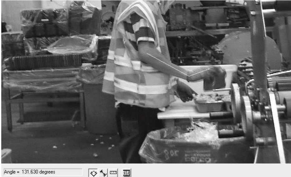
Figure 5 Screen capture during video analysis of wrist angle using MVTA. The yellow lines are placed by analysts on the following landmarks: Olecranon, styloid process of Ulna and dorsal surface of the hand.
