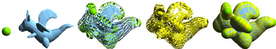
Figure 5.4: Triangle and quadrilateral primitives after culling. From left to right, each picture represents the two models (ball and dragon), triangle primitives after culling (two different colors represent triangles from the two different models), quadrilateral primitives after culling (yellow), and finally the rendered Minkowski sum.
