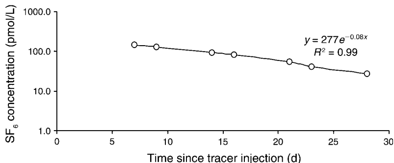
FIG. 8. Mean concentration of SF 6 in Herman Pit as a function of time in days since initial injection on 22 June 1998.
