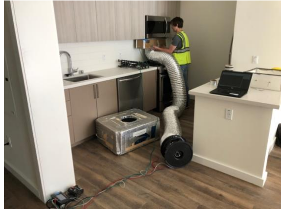
Figure 5. Ventilation grille testing: diagram of the test (left); photo during field testing (right).
