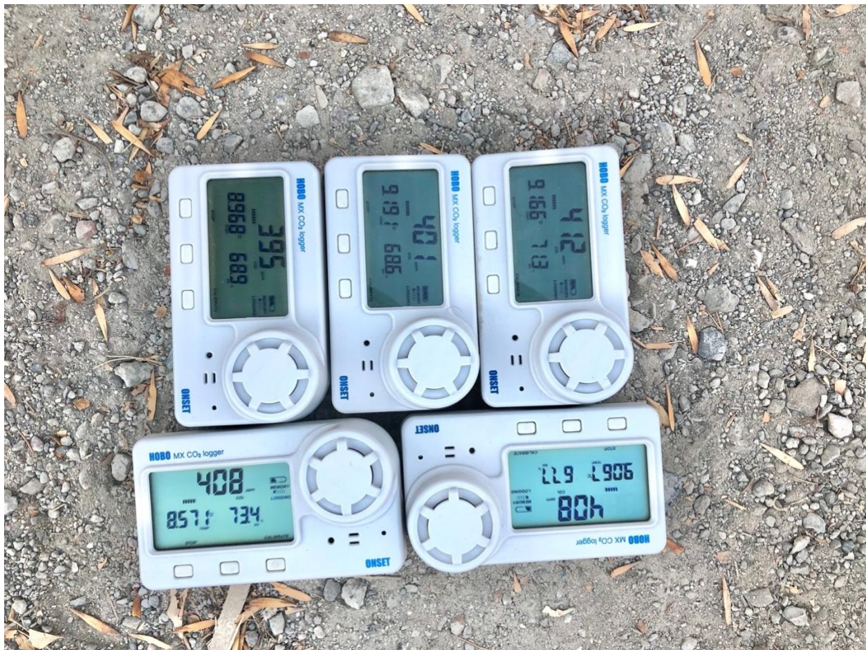
Figure 9. Post-calibration photo of HOBO CO 2 sensors showing they are within +/- 20 ppm (5%) of each other.
