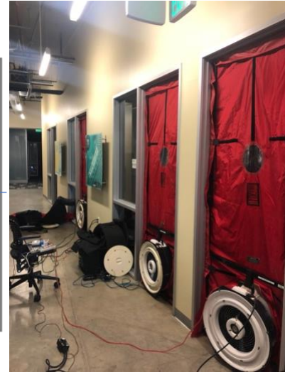
Figure 7. Guarded blower door test: diagram of the test (left); photo of field testing (right).
