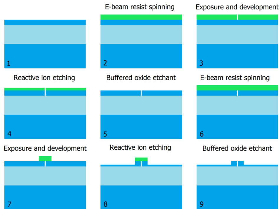
Figure 3.5. Fabrication process for the proposed slot-rib waveguide. In the illustrations, blue corresponds to silicon, light blue corresponds to silicon dioxide, and green corresponds to the electron beam resist hydrogen silsesquioxane (HSQ).
