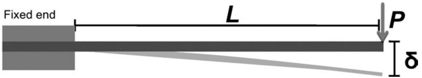
Fig. 3. The fixed-end horizontal deflection cantilever model was used to assess the elastic modulus of the samples. L = length of cantilever, P = force applied to deflect cantilever, \delta = deflection of cantilever.
