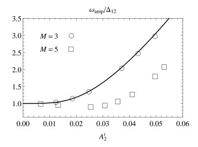
**Figure 3.14**: Plot of the beat frequency of the mode 1 amplitude, as a function of the amplitude of mode 2, for  $k_{\perp} = 10k_1$ . The analytical result is obtained from Eq. (3.330) and depicted in a solid curve. The numerical result for M = 3 and M = 5 are depicted in circles and squares.
