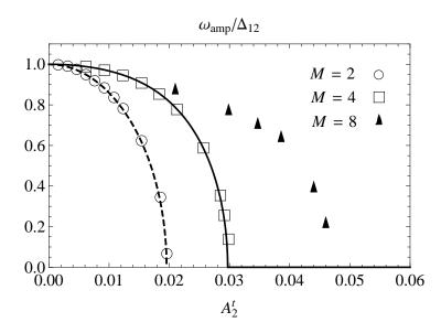
**Figure 3.19**: Beat frequency of the amplitude of mode 1 vs. the amplitude of mode 2, for  $k_{\perp} = 10k_1$ . The analytical result for M = 2, obtained in Eq. (3.286), is depicted in a dashed curve. Analytical result for M = 4 and given by Eq. (3.366), is depicted in a solid curve. Numerical results obtained for M = 2, 4 and 8 number of the present spatial Fourier terms are depicted respectively with circles, squares and triangles.
