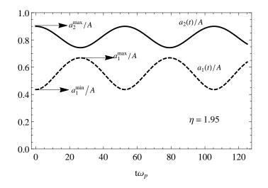
**Figure 3.6**: Plot of  $a_2$  and  $a_1$  vs. time for  $\eta = 1.95$ , for the ratio  $a_1^{\min}/a_2^{\max} = 0.48$ .
