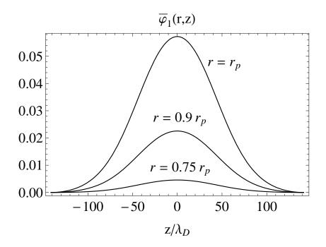
**Figure 1.9**: Plot of the scaled Debye shielded squeeze potential  $\overline{\varphi}_1(r, z)$  as a function of the axial position, at radii  $r = r_p$ ,  $0.9r_p$  and  $0.75r_p$ , for a plasma with the same parameters as Fig. 1.7
