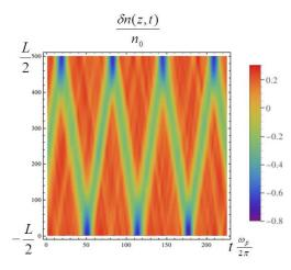
**Figure 4.4**: Plot of the density perturbation of EAW<sub>1</sub> along the plasma as a function of time, in a plasma with  $k_{\perp}L = 18.44$ ,  $L/\lambda = 37.3$ .
