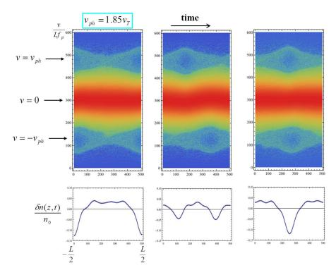
**Figure 4.5**: The three upper plots are density plots of the distribution function f(z, v) of the EAW<sub>2</sub>. Horizontal axis is the position along the plasma from -L/2 to L/2, and the horizontal axis is the particle velocity from  $v = -2.8v_T$  to  $v = 2.8v_T$ . The three lower plots are density perturbations related to the distribution function plots. The physical parameters of the plasma are  $k_{\perp}L = 18.44$ ,  $L/\lambda = 37.3$ .
