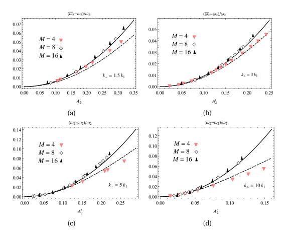
**Figure 3.9**: Plot of the change in mode 2 eigenfrequency of a traveling wave due to the its large amplitude(nonlinearity) for 4 values of  $k_{\perp}/k_1$ . The analytically evaluated frequency obtained from Eq. (3.257) and Eq. (3.35) are depicted respectively in dashed and solid curves. Numerically evaluated results for M = 4, 8, 16 are also depicted.
