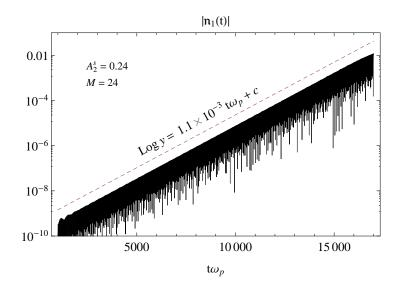
**Figure 3.26**: Plot of  $|n_1(t)|$  vs. time, for  $k_{\perp} = 10k_1$  and  $|A_2^s| = 0.24$ . The plasma was driven by the potential  $\overline{V}_2 = 1 \times 10^{-4} m_q (\omega_p L/2\pi)^2$  for a forcing time  $T_F \omega_p = 180$ .
