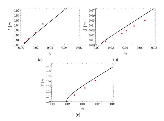
**Figure 4.8**: Exponential growth rate of small amplitude EAW<sub>1</sub> in the presence of large amplitude EAW<sub>2</sub>. Solid curves are obtained from Eq. (4.57). Physical parameters related to the plot are (4.8a): $k_{\perp}L = 15$ ,  $L/\lambda = 44.5$ , (4.8b): $k_{\perp}L = 19.5$ ,  $L/\lambda = 45.9$ , (4.8c): $k_{\perp}L = 18.44$ ,  $L/\lambda = 37.3$
