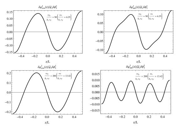
**Figure 1.1**: The change to the spatial dependence of mode potential for mode m = 1, with  $\cos(\omega_r t)$  and  $\sin(\omega_r t)$  time dependence, in a plasma with  $k_{\perp}L = 15\pi$  and scaled plasma frequencies  $\omega_p/k_1v_T = 90$  and  $\omega_p/k_1v_T = 200$ , corresponding to mode phase velocities  $\omega_{r_0}/k_1v_T = 6.25$  and 13.42 respectively.
