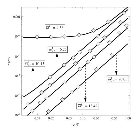
**Figure 1.3**: Mode damping rate vs. size of the squeeze potential  $\varphi_s/T$ , for phase velocities:  $\omega/k_1v_T = 4.56, 6.25, 10.13, 13.42$  and 20.03 for the mode m = 1. Analytically calculated damping rates are shown in solid black lines. Computer simulation results are shown with diamonds.
