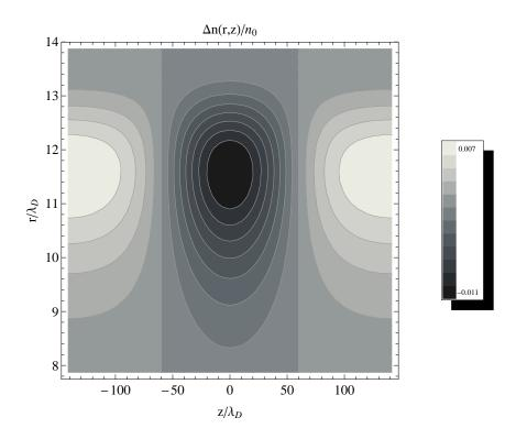
**Figure 1.8**: Contour plot of the difference between the squeezed equilibrium density and the unsqueezed equilibrium density (the latter is the same as Fig. 1.7) as a function of the radial and axial positions for a plasma, for a squeeze with  $\Delta = 2.86$ cm and  $\varphi_{sq} = 0.1$ eV.
