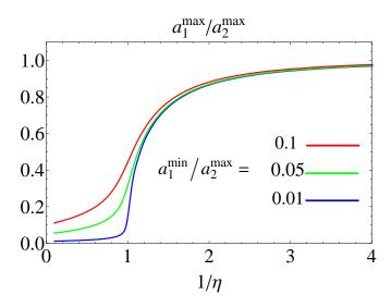
**Figure 3.8**: Plot of the maximum value the amplitude of mode 1 reaches  $(a_1^{\text{max}})$  from a minimum  $(a_1^{\min})$ , as a function of the parameter  $\eta$ , for initial conditions such that mode 2 is dominant, i.e.  $a_1^{\min}/a_2^{\max}$  is small.
