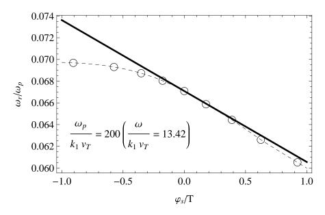
**Figure 1.2**: The real part of the mode frequency  $\omega_r/\omega_p$  vs. the size of the Debye shielded squeeze potential  $\varphi_s/T$  for mode m = 1, where  $\varphi_s \equiv \varphi_1(0)$ , for  $\omega_p/K_1V_T = 200$  (which implies  $\omega_{0r}/K_1V_T = 13.42$ ). Analytically calculated results, shown here with a solid line, are up to the first order in  $\varphi_s/T$  using Eq. (1.71); computer simulation results are shown with circles.
