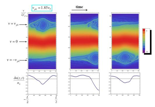
**Figure 4.3**: The three upper plots are density plots of the distribution function f(z, v) of the EAW<sub>1</sub>. Horizontal axis is the position along the plasma from -L/2 to L/2, and the horizontal axis is the particle velocity from  $v = -2.8v_T$  to  $v = 2.8v_T$ . The three lower plots are density perturbations related to the distribution function plots. The physical parameters of the plasma are  $k_{\perp}L = 18.44$ ,  $L/\lambda = 37.3$
