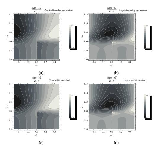
**Figure 2.6**: Contour plots of the real and imaginary part of  $\delta f$  in the *z*, *v* phase-space, near the separatrix ( $v/v_s \approx 1$ ), for  $v_T/v_s = 1.73$  and for diffusion coefficient  $DL/v_s^3 = 2 \times 10^{-4}$ . Plots (2.6a) and (2.6b) are obtained from the analytical boundary layer method and plots (2.6a) and (2.6b) are obtained from the numerical grids method.
