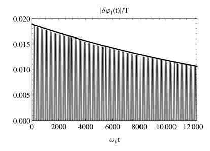
**Figure 1.5**: The  $m_z = 1$  Fourier component  $\delta \varphi_1(t)$  of the space-charge potential  $\varphi_p(z,t)$  and the exponentially damping amplitude  $g(t) = 0.0188 \exp[-4.7 \times 10^{-5}(\omega_p t)]$  (thick curve), obtained by fitting to  $\delta \overline{\varphi}^1(t)$ , as functions of time.
