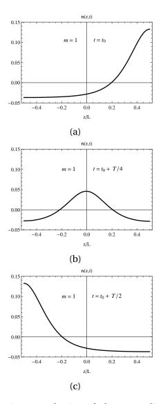
**Figure 3.2**: Plots of the density perturbation of a large amplitude nonlinear standing mode m = 1, for  $k_{\perp} = 10k_1$ , obtained from fluid simulations described in appendix F, with M = 26.
