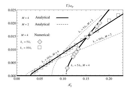
**Figure 3.23**: Growth rate of mode 1 vs. the amplitude of mode 2. The analytical growth rate for M = 4, which is  $\Gamma$  defined in Eq. (3.368), is depicted in a solid curve, numerical result for M = 4 is depicted in squares for  $k_{\perp} = 10k_1$  and diamonds for  $k_{\perp} = 5k_1$ ; and for comparison the analytical result for M = 2, given by Eq. (3.288), is depicted in dashed curves.
