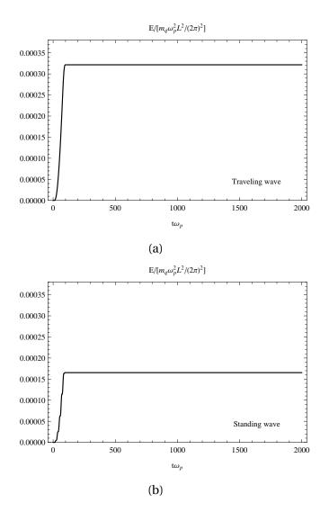
**Figure 3.4**: Figure (3.4a) shows the energy of a traveling wave of amplitude  $A_2^t = 0.24$  and Fig. (3.4b) shows the energy of a standing wave of amplitude  $A_2^s = 0.24$ . Forcing time was  $T_F \omega_p = 97$  and drive potential was  $\overline{V}_2 = 1.8 \times 10^{-4} [m_q \omega_p^2 (L/2\pi)^2]$  and M = 8 Fourier terms were kept, for  $k_{\perp} = 10k_1$ .
