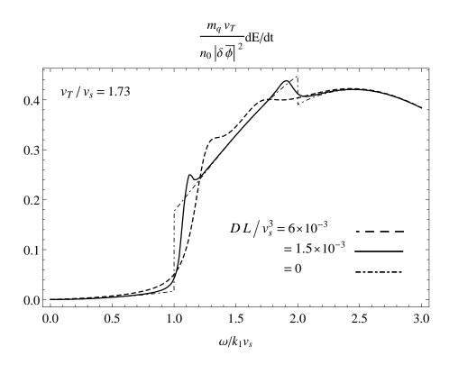
**Figure 2.9**: Heating per unit time as a function of  $\omega$ , obtained from numerical grids method for  $D = 1.5 \times 10^{-3}$ , and  $D = 6 \times 10^{-3}$ , and obtained from Eq. (2.42) for D = 0.
