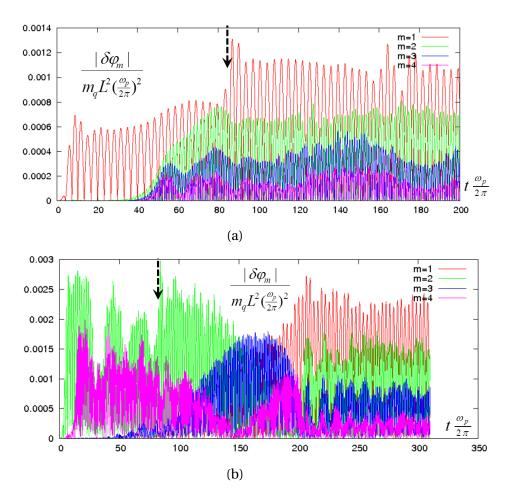
**Figure 4.1**: Amplitudes of the first four spatial Fourier components, m = 1, 2, 3 and m = 4, as a function of time. In figure (4.1a) external drive potential is  $\cos[k_1z]$  to excite EAW<sub>1</sub>. In figure (4.1b) external drive potential is  $\cos[k_2z]$  to excite EAW<sub>2</sub>. Dashed arrow shows the point in time where the drive is turned off. The physical parameters of the plasma are  $k_{\perp}L = 18.44, L/\lambda = 37.3$
