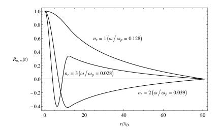
**Figure 1.10**: Plot of the radial dependence of the modes  $\mu = (n_r, m)$ , with axial mode number m = 1 and three radial mode numbers  $n_r = 1, 2, 3$ , in an unsqueezed plasma with the same parameters as Fig. 1.7.
