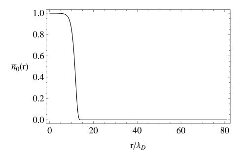
**Figure 1.7**: Plot of the equilibrium density for a plasma with T = 50 meV,  $L = 10 \text{cm}(L/\lambda_D = 282.6)$ ,  $\omega_p = 1.263 \times 10^6 \text{Rad/s}$ ,  $r_p \approx 0.42 \text{cm} (r_p/\lambda_D \approx 11.87)$ ,  $r_w = 2.86 \text{cm}(r_w/\lambda_D = 80.83)$ . Maximum density of the plasma at r = 0 is normalized to 1.
