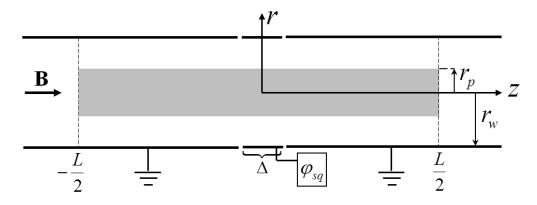
**Figure 1.6**: Schematic depiction of the trap geometry and squeeze potential  $\varphi_{sq}$  applied to a cylindrical sector of width  $\Delta$ . Other parts of the trap wall are grounded. Particles are assumed to reflect at the axial ends  $z = \pm L/2$ .
