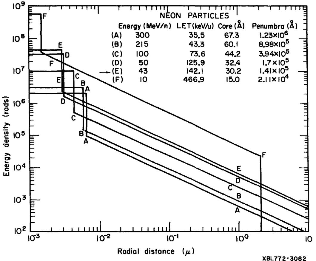
Figure 2. Diagram to show core regions and penumbra regions for tracks of neon particles at various energies. The core energy densities are to the left of the vertical discontinuity, and the penumbra energy densities are to the right. Each discontinuity is about 20 rads. Diagram reproduced from Magee and Chatterjee, 1977.
