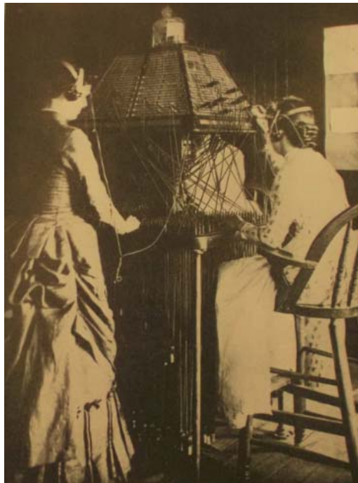
An early “lamp-shade” or “pyramid” switchboard from around 1882. 499
