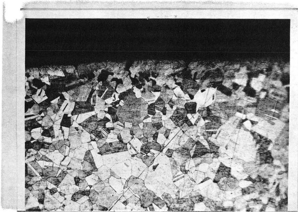
Fig. 41 - Extensive recrystallization .005 to .007 in. into the surface of Inconel electrodes.
