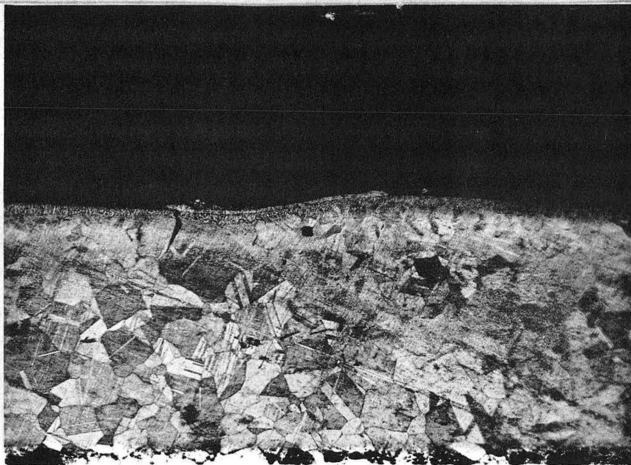
Fig. 43 - Mechanical bond of material transferred across the gap as a result of a spark. Inconel.
