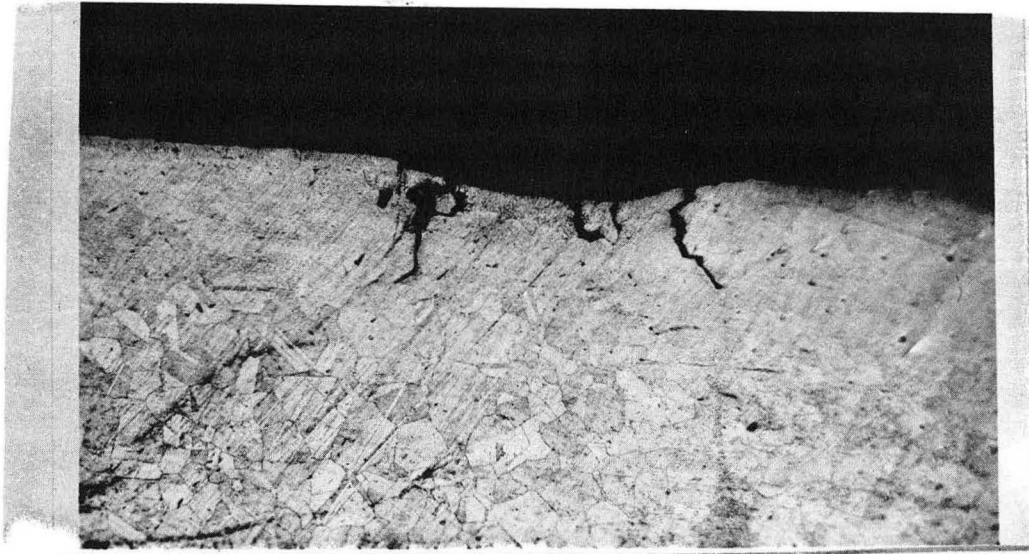
Fig. 40 - Spark crater .025 in. in diameter. Inconel Electrodes. Note .002 - .008 in. radial cracks.
