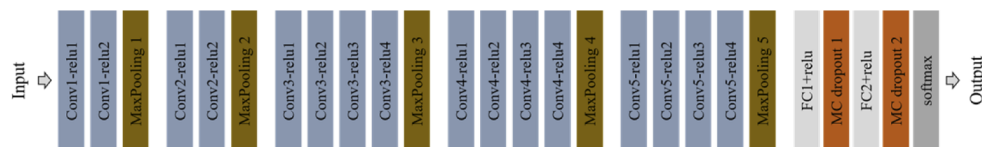
Fig. 2. Structure of our BNN architecture (VGG19 as baseNet).
