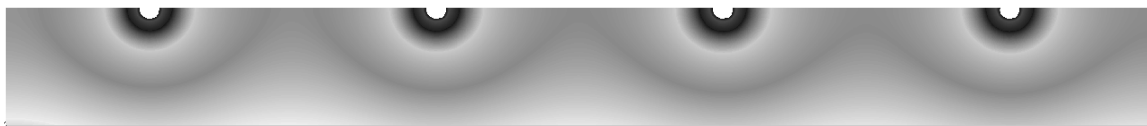
Figure 13c: Isothermal contours as graduated colored/grayscale fills provide a visualization of continuous temperature gradients throughout a cross-section of the chilled slab material.
