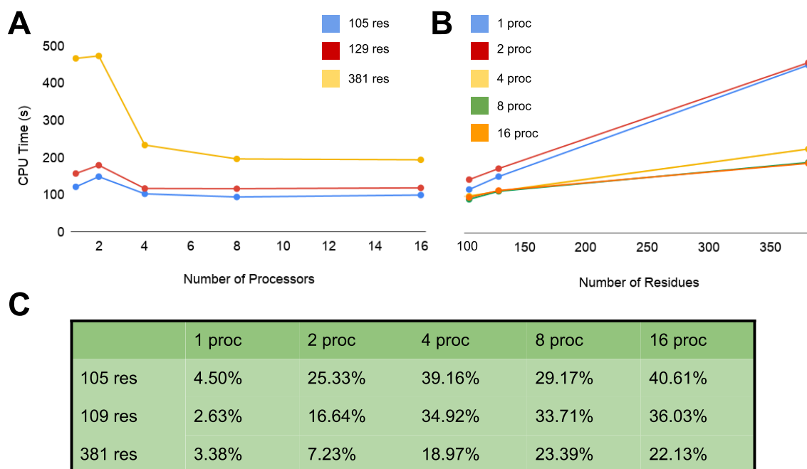
Figure 4.4. Computational resource scaling benchmark of Titr-DMD, plotted by (A) the number of processors and (B) the number of residues. Note the linear scaling with number of residues and that good performance is reached with four processors. (C) The percent increase of time for Titr-DMD over unmodified DMD. Note that the increase is relatively small and only becomes significant with many processors as the time DMD takes shortens.
