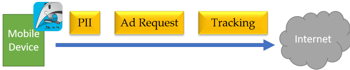
Figure 1.1: Overview of contributions of this thesis. First, we build AntMonitor – a system for efficient traffic interception on a mobile device (Sec. 1.2.1). Next, we apply AntMonitor to different tasks: (i) detecting and preventing PII exposure (Sec. 1.2.2); (ii) detecting and blocking ads (Sec. 1.2.3); and (iii) detecting and blocking third-party trackers (Sec. 1.2.4).
