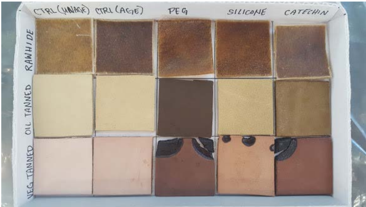
Fig. 3. Appearance of aged samples (post-treatment) with aged and unaged controls.
