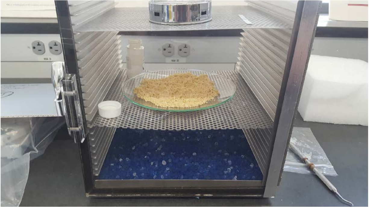
Fig. 4. Setup for desiccation of catechin hydrate.
