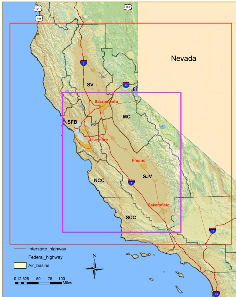
Figure 1: The outer red rectangle shows the CCOS domain, modelled on a 190 x 190 grid. The inner purple rectangle shows the extent of the 96 x 117 SARMAP domain. Labeled air basins include Sacramento Valley (SV), San Joaquin Valley (SJV), South Central Coast (SCC), North Central Coast (NCC), San Francisco Bay Area (SFB), Mountain Counties (MC), and Lake Tahoe (LT).
