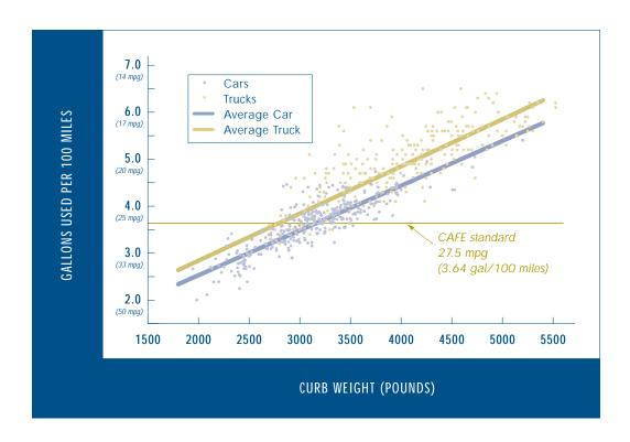
Note that car weights and truck weights have been increasing over the past decade despite strong counteracting pressure from CAFE. Furthermore, the profit margin associated with large vehicles has traditionally been much higher than that associated with small ones. Thus there are substantial market incentives for manufacturers to increase vehicle weights and no restraints on them doing so once CAFE is removed.
