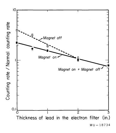
Fig. 4. Effect of the electron filter as a function of the thickness of lead in the filter. The normal operating condition (2 in. of Pb, magnet on) is taken as 1.0 on the ordinate.
