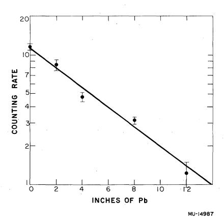
Fig. 13. Counting rate vs thickness of lead absorber, showing the exponential decay, the slope of which gives the cross section.
