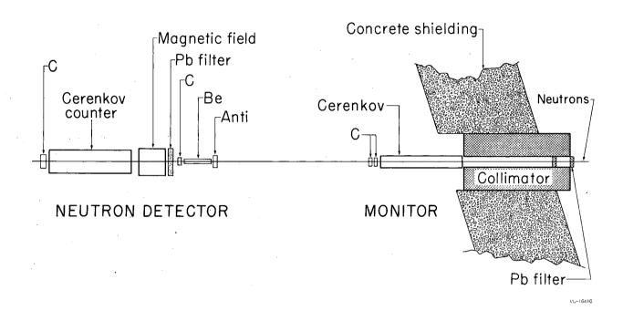
Fig. 2. Experimental arrangement (schematic representation), showing the collimator, monitor telescope, and neutron-detector telescope.
