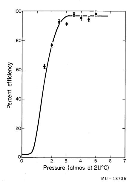
Fig. 7. Measured detection efficiency of CCl<sub>2</sub>F<sub>2</sub> Cerenkov counter vs gas pressure for 3-Bev pions. The curve was taken with 1950 volts on the photomultiplier tube.
