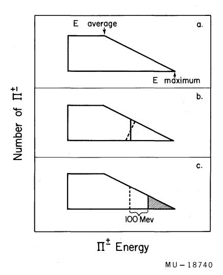
Fig. 12. Simplified pion-energy spectrum used to derive the effective neutron-energy spectrum.
