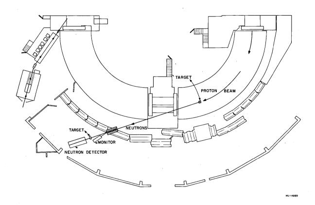
Fig. 1. Path of the neutron beam from the Bevatron through the detector. This shows the original monitor.
