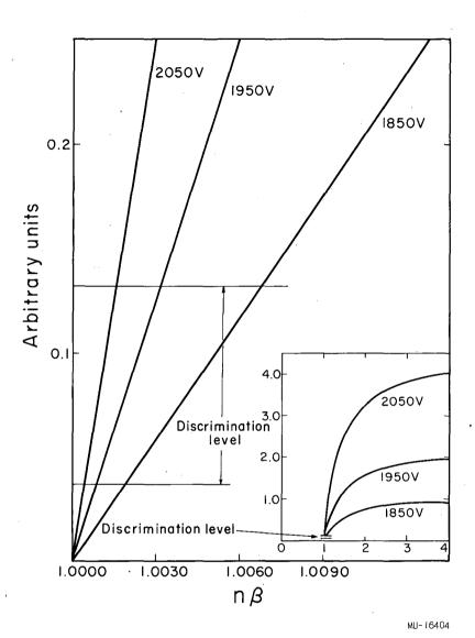
Fig. 9. Output voltage of phototube,  $V_g$  -  $A_g$  [1 -  $(1/n^2\beta^2)$ ] vs n $\beta$ . The horizontal line corresponds to an output voltage of 2 v for a detection efficiency of 90%.
