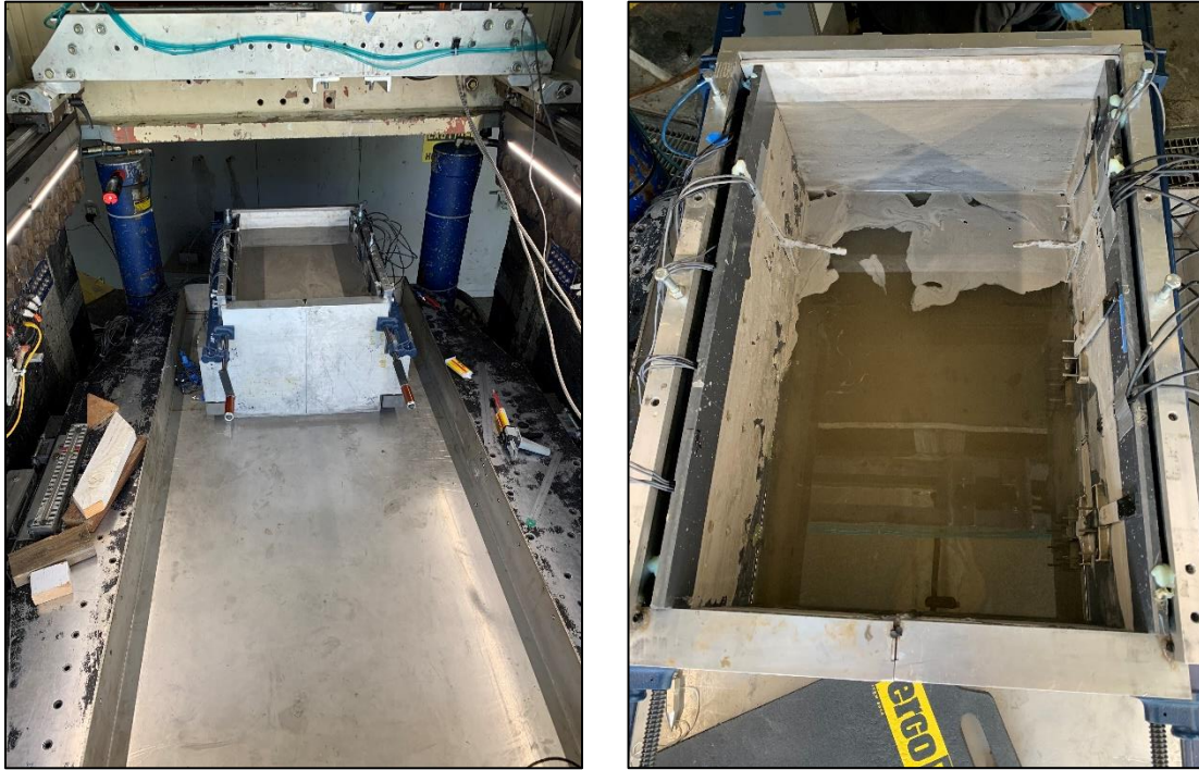
Figure 15. Left: Ash lift poured in container. Right: Excess water removed before pouring lift.
