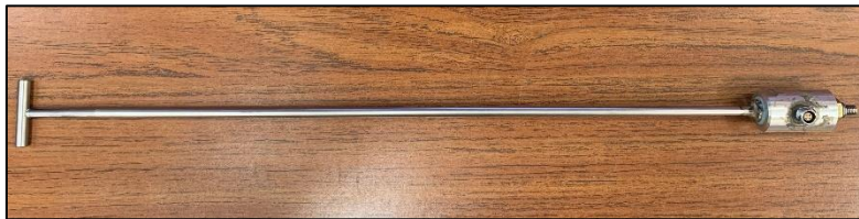
Figure 31. T-bar penetrometer used for 1 g tests.
