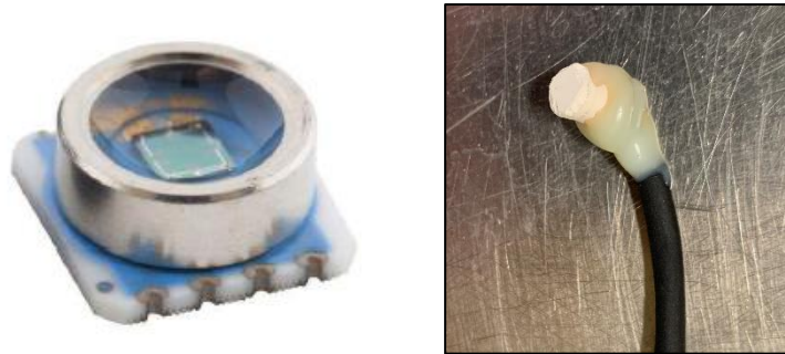
Figure 19. Left: miniature SMD pressure sensor (MS5407-AM, Intersema 2007). Right: constructed tensiometer for FR06.
