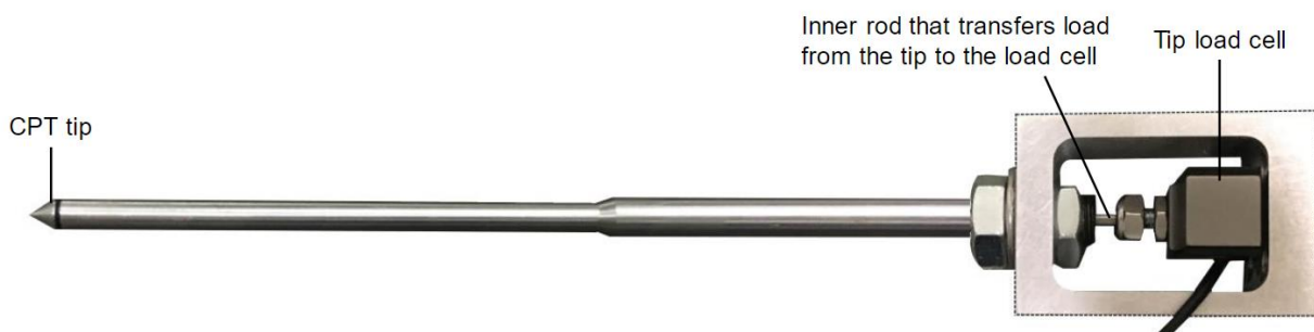
Figure 18. Miniature CPT probe used for centrifuge testing (EPRI 2021).
