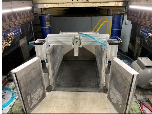
Figure 30. Modified fly ash impoundment model for 1 g tests.
