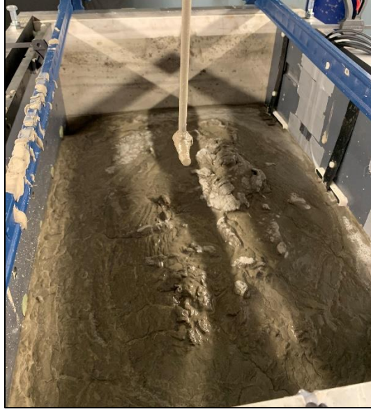
Figure 86. Uneven ash surface formed during specimen preparation for T2.
