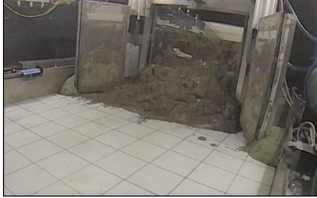
Figure 38. Initial slope instability failure during FR06.
