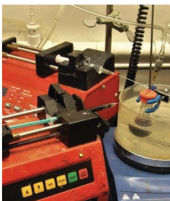
Figure 3-5: Photograph of experimental setup employing parallel slow addition.
