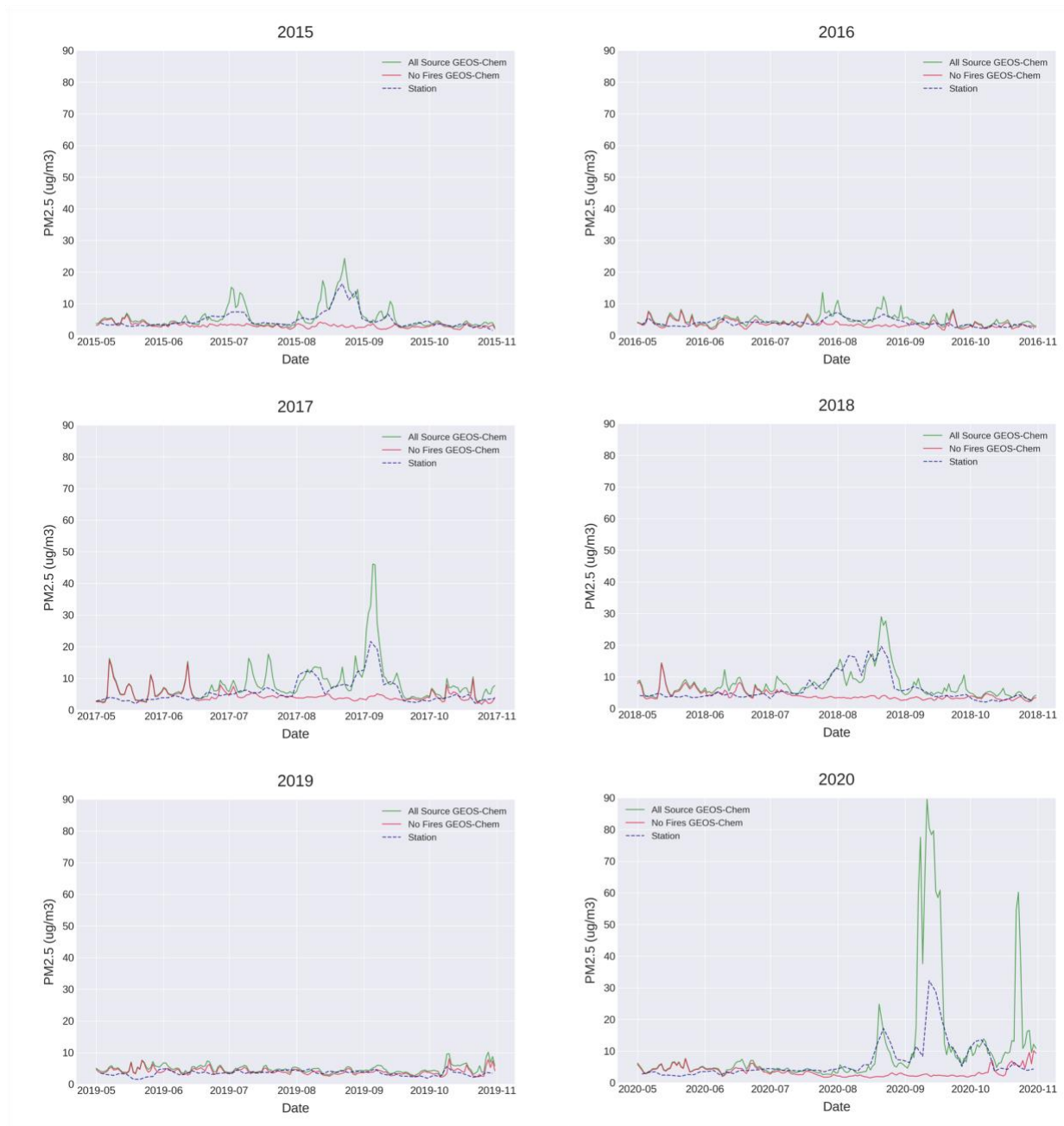
Figure B 4: We create time-series data for modeled PM 2.5 by averaging values from the IMPROVE monitoring stations within each GEOS-Chem cell. IMPROVE data is available every three days, hence we obtain daily model estimates every three days which are then averaged to obtain a single daily average for the entire region. To ensure data consistency, we include measurements from stations that provided data for at least 50% of the three-day measurements in each of the six years of the study period.
