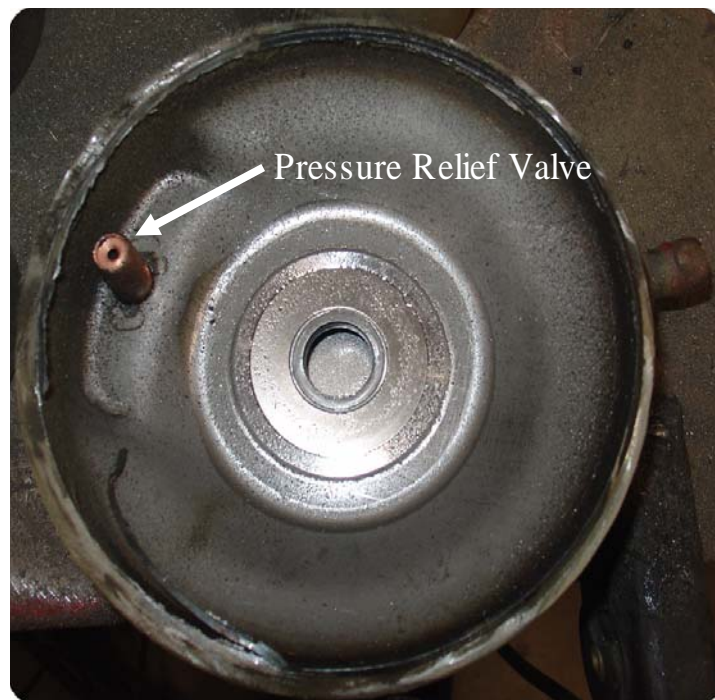
Figure 7 Pressure Relief Valve
