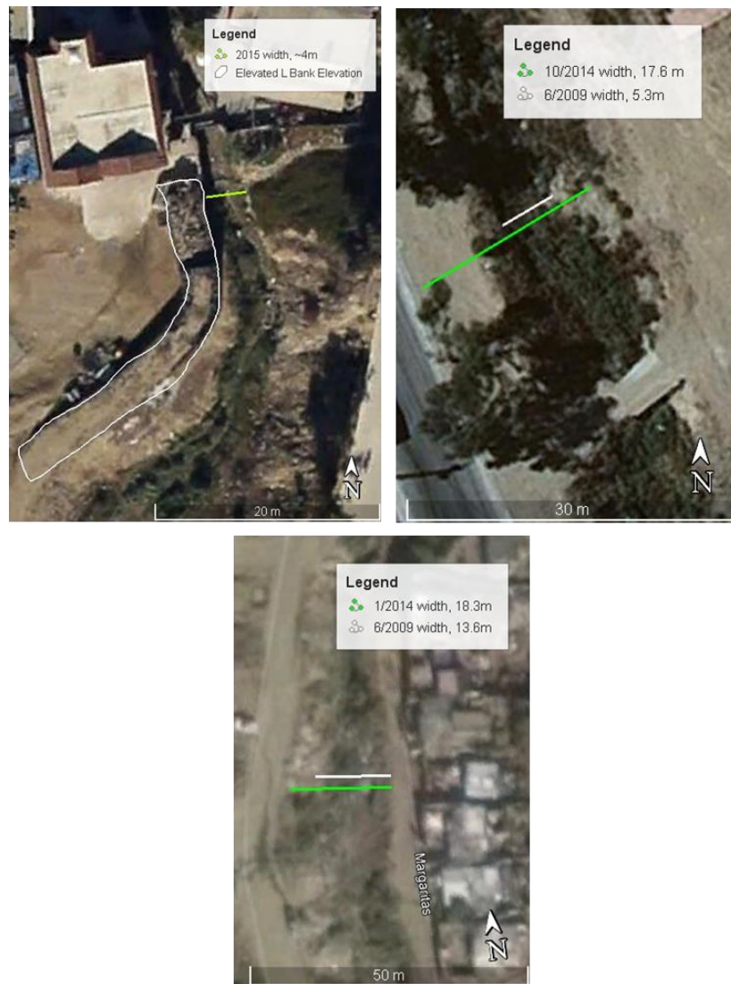
Figure 3. Color aerial imagery indicating channel width for a) Main8, b) SEC107, and c) SW305. Although surveyed bankfull width in 2014 at Main 8 was estimated to be 12 m, 2015 aerial imagery indicates that bankfull width was ~4m. Bankfull width in 2014 was incorrectly estimated because it was based on matching the top elevation a structure on the left bank (white polygon), which was artificially raised, to the right bank elevation. At SEC107 and SW305, change in width from aerial imagery validates that there was approximately 12 m (SEC107) and 5 m (SW305) of widening.
