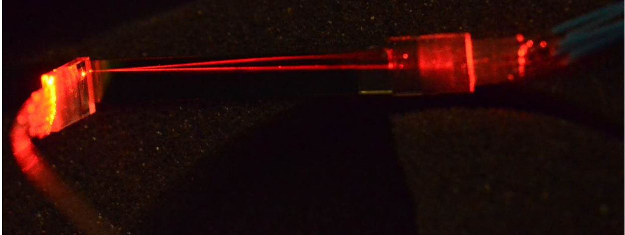
Figure 8.7: An image of the device chip with fiber optics attached, and light scattering towards the exit fiber optics.
