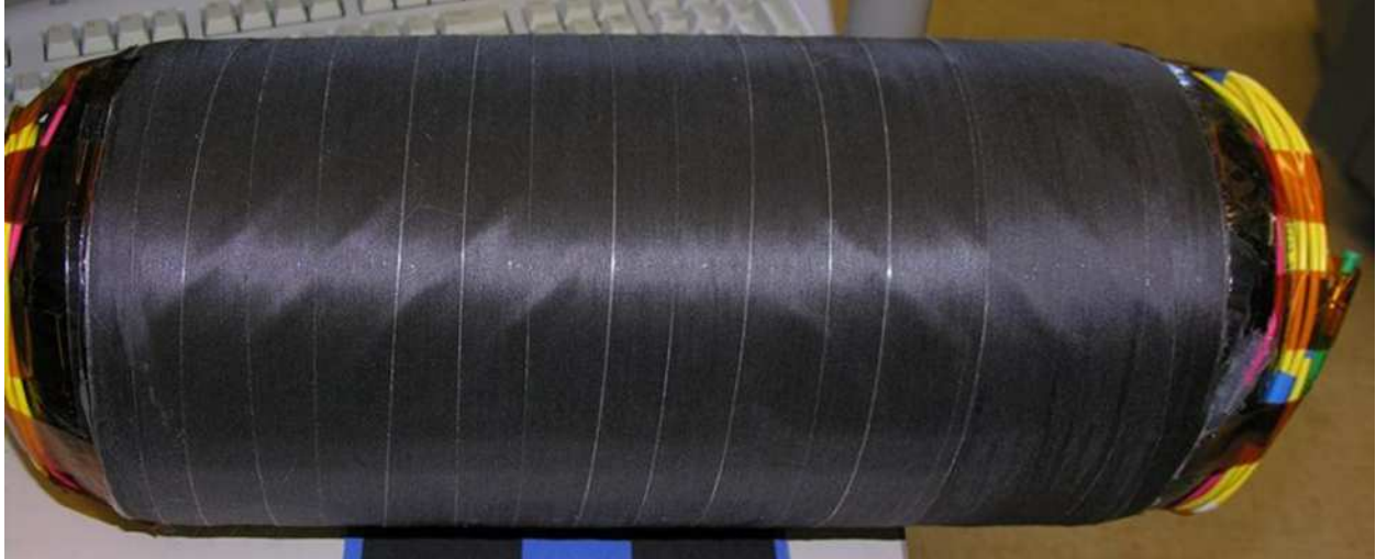
Figure 3.3: COPV with first layer of sensing fibers, over-wrapped with a layer of composite. The glare from an overhead light highlights the 45° runs' ridges from the epoxy holding the now-embedded fiber optics in place.
