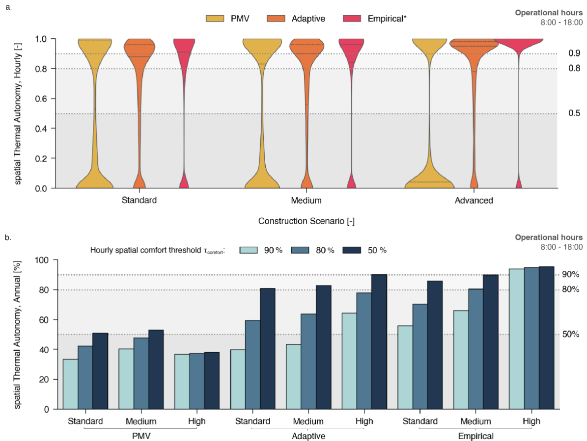
Figure 4: a) Hourly sTA distributions using PMV, adaptive, and empirical models for different passive design levels and medium zone size: adaptive and empirical model tend to predict higher sTA_{hourly} and are more sensitive passive design measures; b) Annual sTA comparison across comfort models for varying hourly spatial thermal comfort thresholds \tau_{comfort} : adaptive and empirical model consistently predict higher sTA_{annual} than PMV, independent of chosen \tau_{comfort} .
