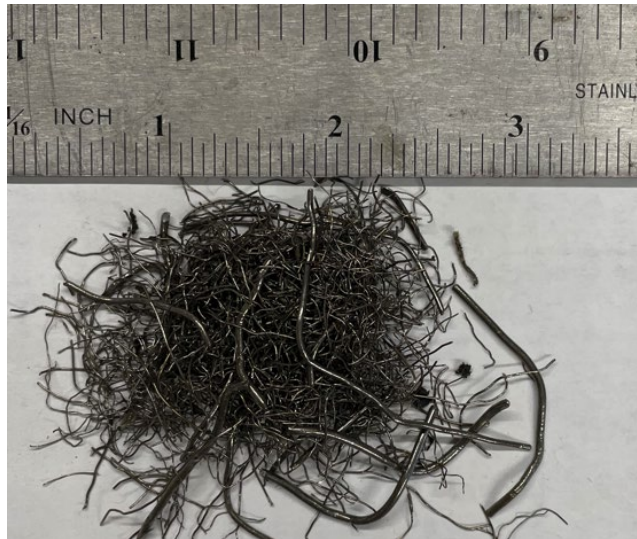
Figure 5.8: Sample of COR-TUF UHPC recycled steel fibers.
