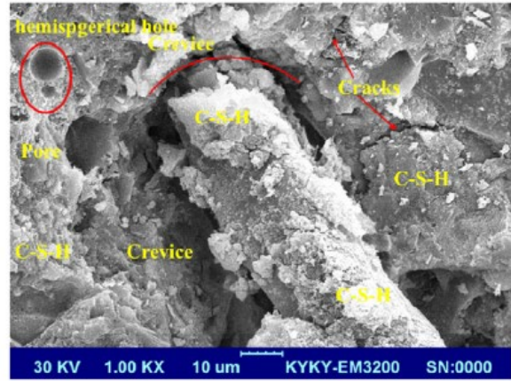
(b) CTF reinforced concrete
