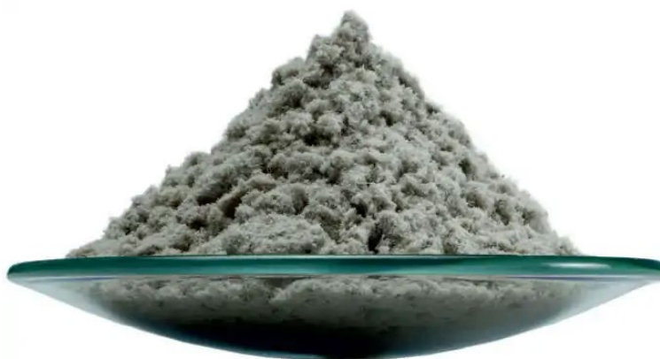
Figure 4.7: ROAD-CEL cellulose fiber produced by J. Rettenmaier USA LP.
