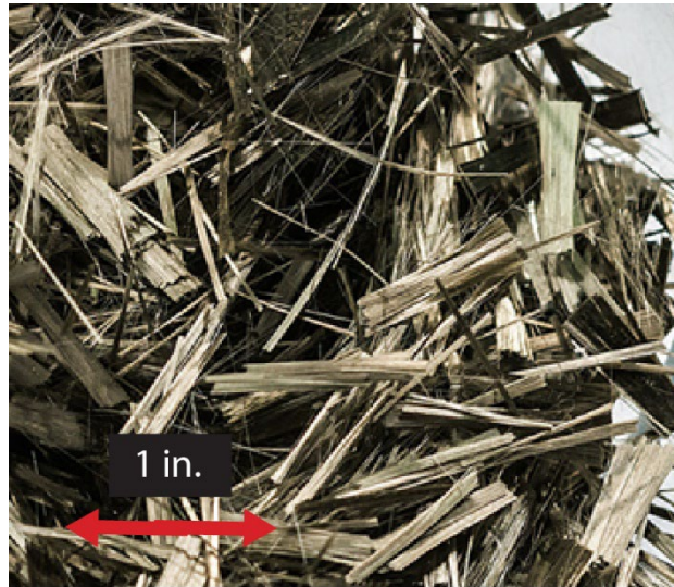
Figure 7.5: Basalt fibers by Technobasalt.
