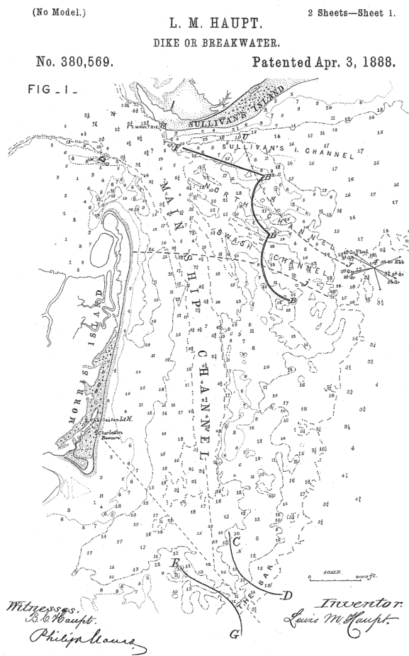
Figure 14 Lewis M. Haupt's patent for the reaction breakwater shows his invention sited at the entrance to Galveston Bay, in the Delaware River, and at the entrance to the Charleston Harbor (US Patent 380569). The breakwater was designed to maintain navigable
