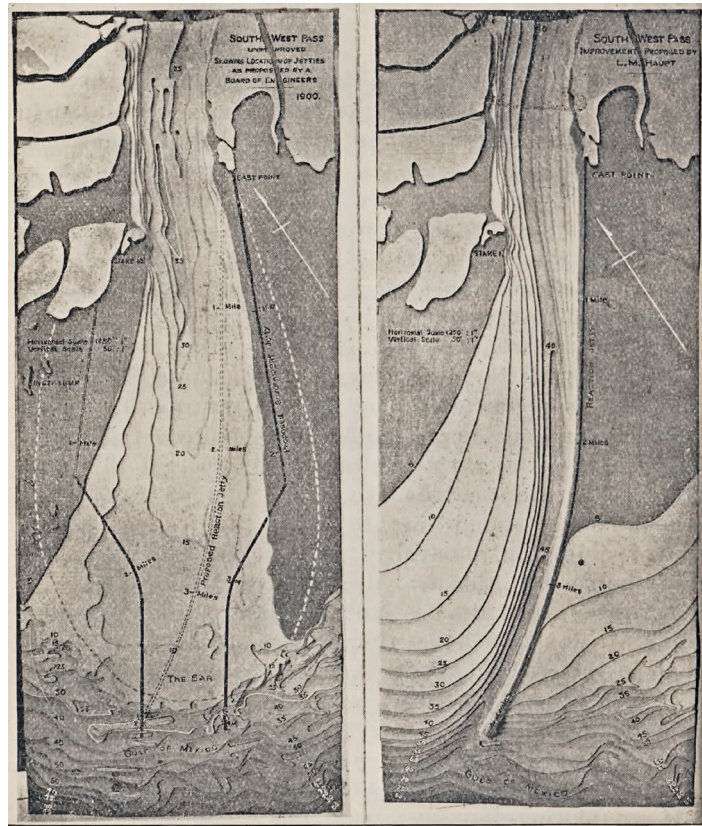
Figure 15b Lewis M. Haupt's topographical models for the Southwest Pass of the Mississippi comparing the USACE plan requiring dredging (left) to his plan using the reaction breakwater without dredging (right). Notice the depth of the channel and deposition of sediment on the western bank. (Source: Lewis M Haupt, 'The Reaction Breakwater as Proposed for the Opening
