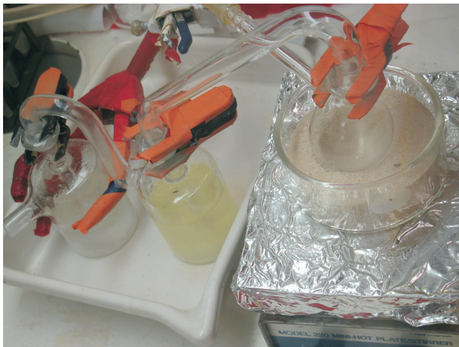
Figure 2.1 The boiling/scrubbing apparatus used to prepare ^{242}\text{Pu} solutions.
