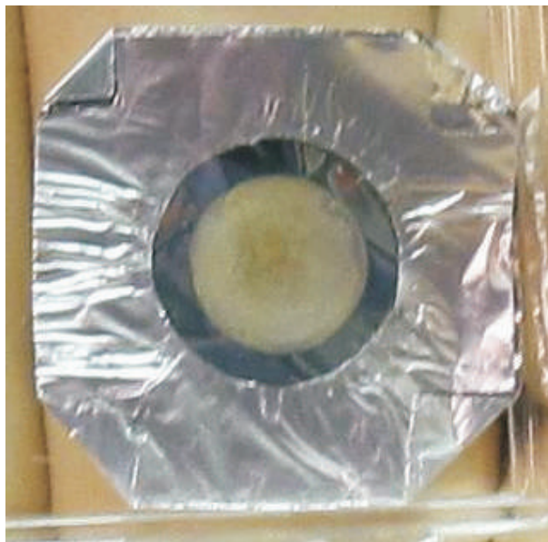
Figure 2.10 Photograph of deposited and baked 6-mm-diameter ^{242}\text{Pu} target on thin Ti wrapped in Al support foil.
