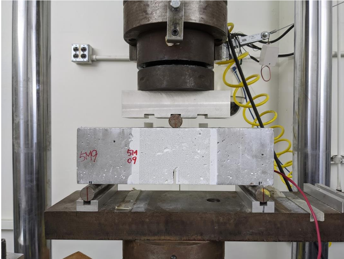
Figure 3-23. The three-point bending test setup with the servo-hydraulic machine and the prismatic concrete specimen.
