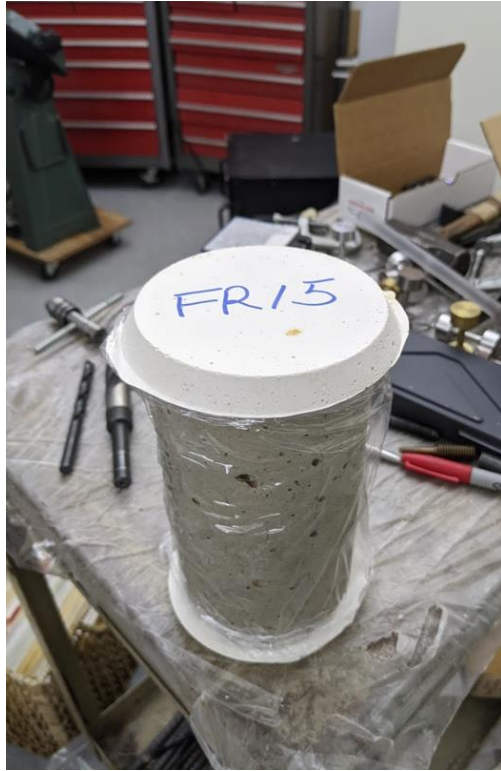
Figure 3-21. The capping of concrete cylinders using hydro-stone gypsum cement.
