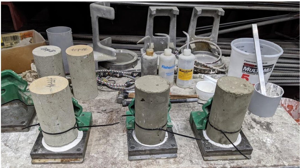
Figure 3-22. The capping process in the structural laboratory.
