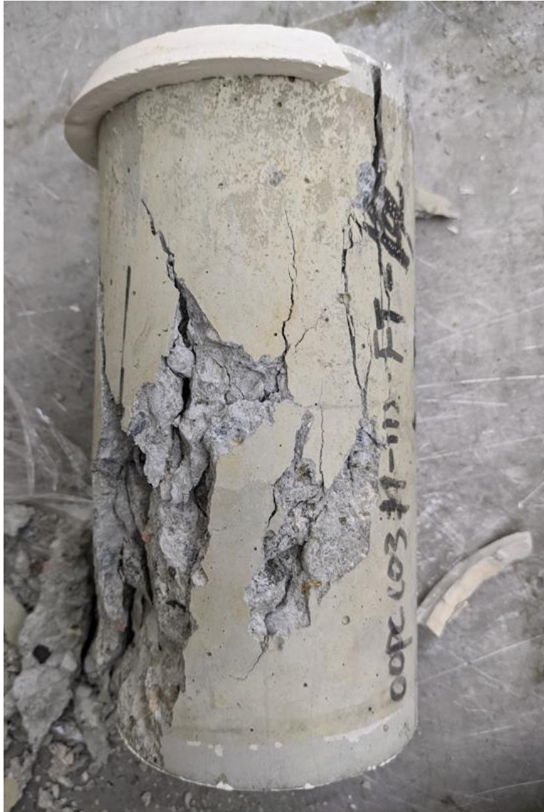
Figure 4-9. The fracture pattern for a plain concrete after compression test.
