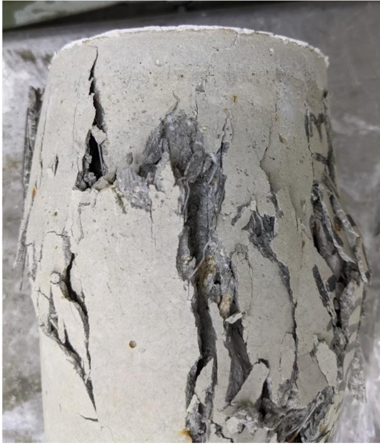
Figure 4-10. The fracture pattern for a fiber-reinforced concrete after compression test.
