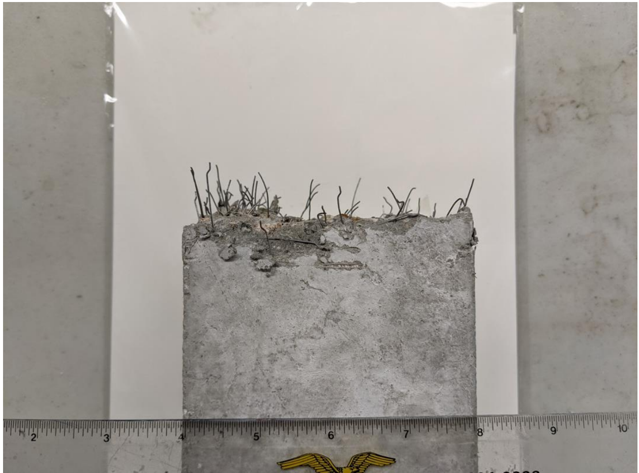
Figure 5-24. The top view of failure of the fiber-reinforced concrete without PCM (HFRC) tested by three-point bending.
