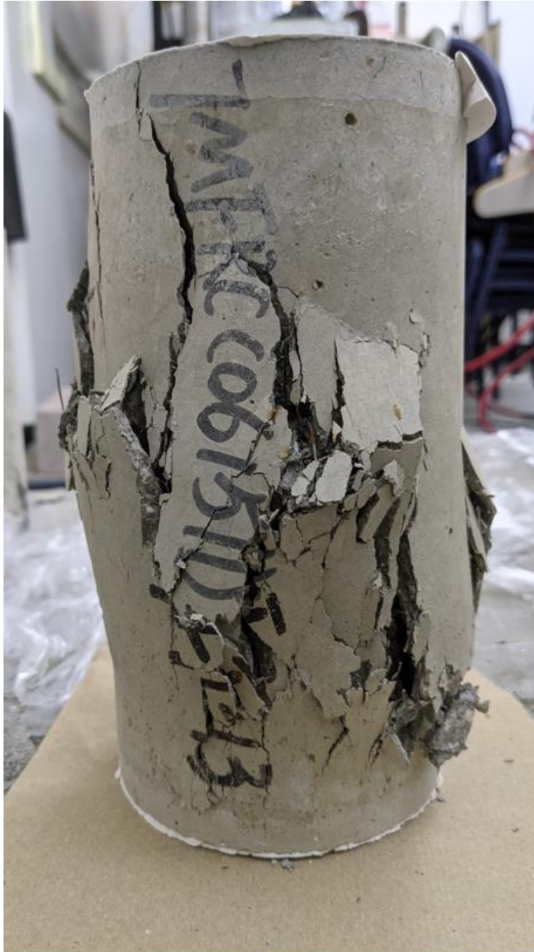
Figure 4-12. The fracture pattern for a fiber-reinforced concrete with 7% PCM after compression test.
