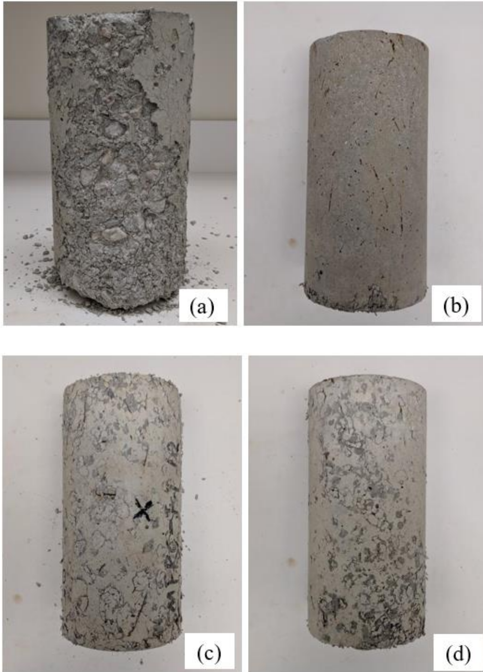
Figure 4-2. Surface conditions after the 30 cycles of freeze-thaw exposure: (a) plain concrete, (b) hybrid fiber-reinforced concrete, (c) hybrid fiber-reinforced concrete with a 5% PCM content, and (d) hybrid fiber-reinforced concrete with a 7% PCM content.
