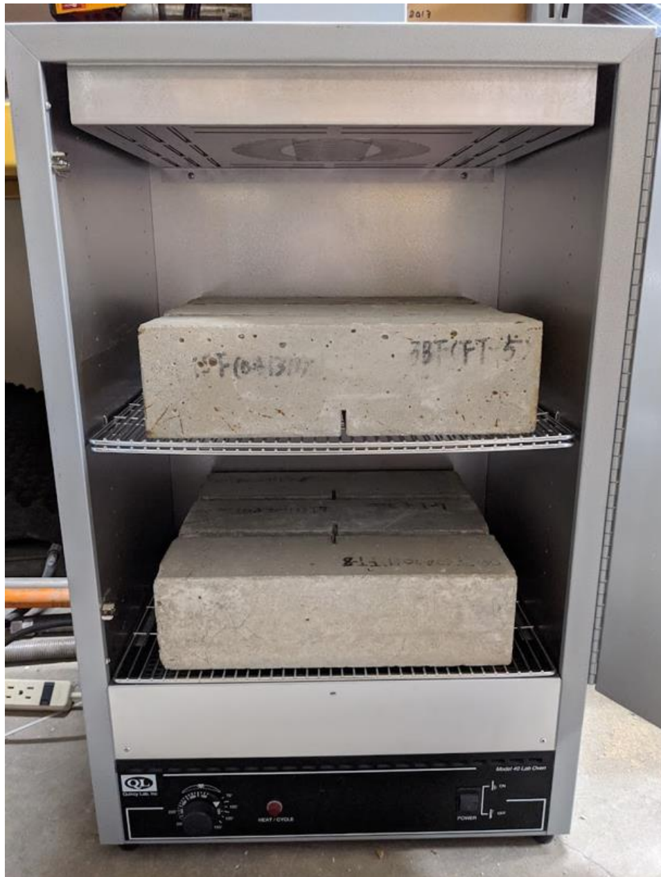
Figure 5-10. The oven used to prepare the concrete specimens for the absorption capacity measurements.
