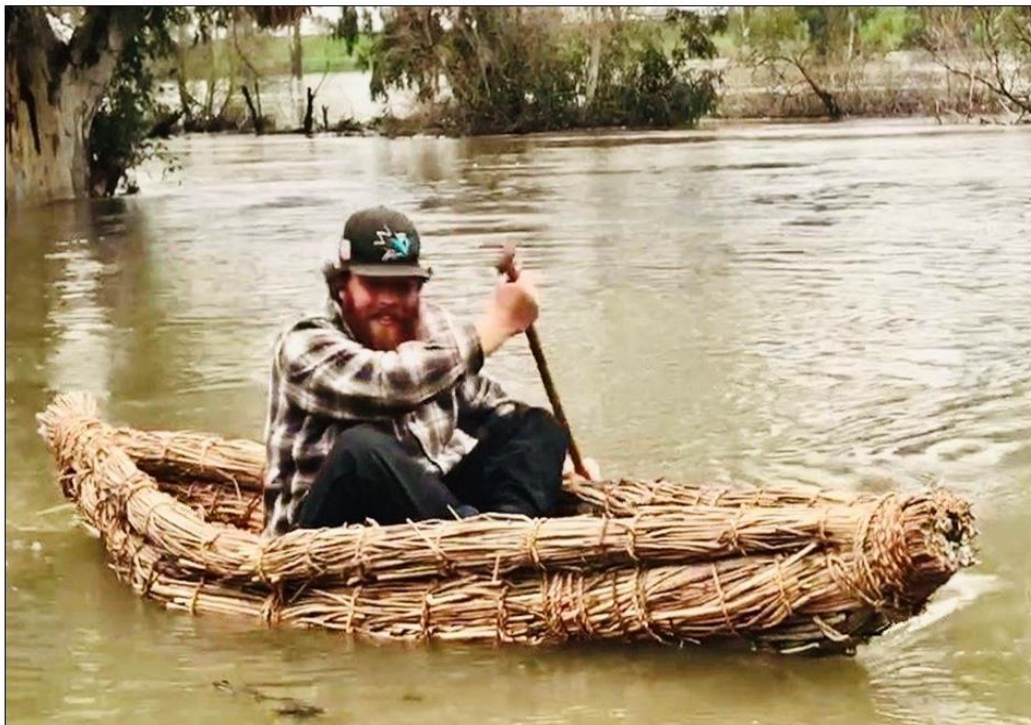
Figure 26. Martijn Kuypers testing the tule boat in Davis, California.
