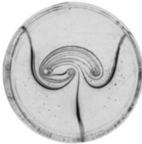
Fig 4.1) Three-rod stirring experiment showing exponential stretching of the fluid material. (Reproduced from Boyland, 2000 with permission ©Cambridge University Press)
