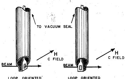
LOOP ORIENTED ( FOR SIGMA TRANSITIONS (  $\Delta m_F = 0$  )
