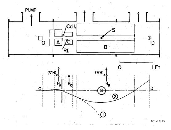
Fig. 3. Schematic diagram of atomic-beam trajectories.
