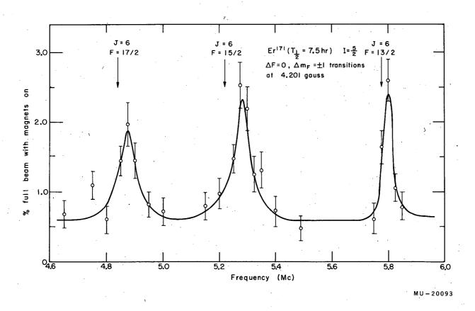
Fig. 36. Resonances in the three highest F states of  $Er^{171}$ .
