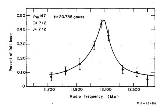
Fig. 17. Promethium-147 resonance curve at 20.755 gauss.
