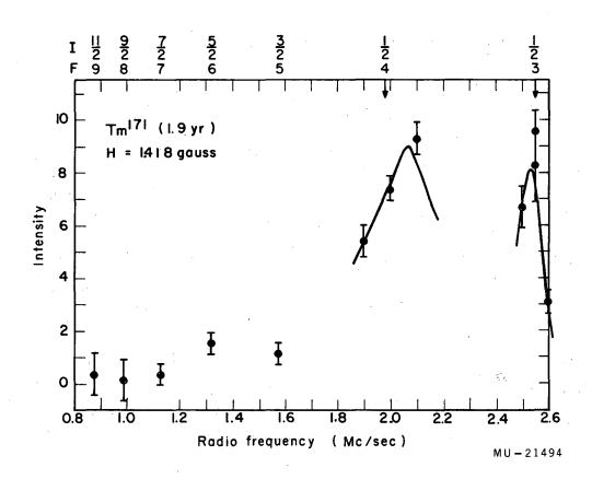
Fig. 35. Identification of the nuclear spin of  $\mathrm{Tm}^{171}$ .
