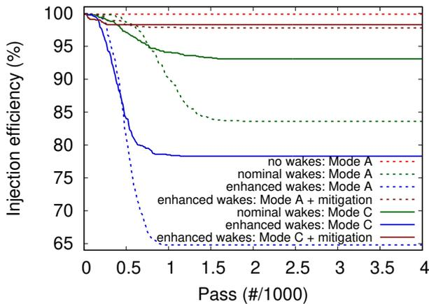
FIG. 13. Capture efficiency as a function of number of passes around the ring after injection, comparing Mode A, where the kicker settings are optimized without including wake field effects, to Mode C, which uses an alternative set of kicker strengths which is more tolerant to wake fields and also changes the injection beta function. Results are shown with and without wake fields, for enhanced wake fields, and for additional mitigations.
