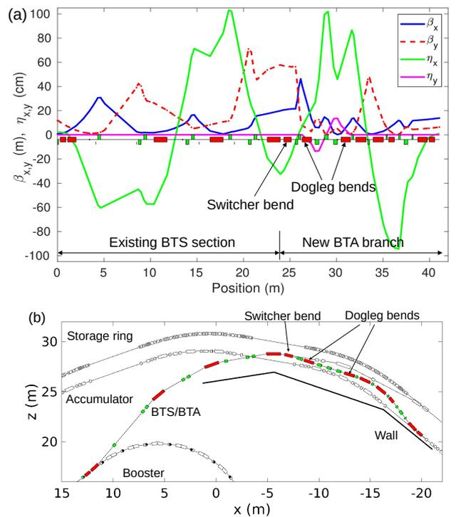
FIG. 6. Twiss functions (a) and layout (b) of the BTA transfer line.
