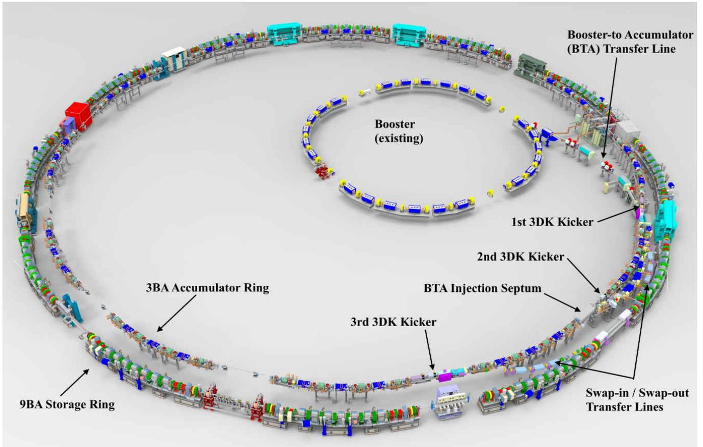
FIG. 1. The Advanced Light Source Upgrade complex. The 3 dipole kickers and injection septum of the 3DK booster-to-accumulator injection scheme are highlighted. Every 1.4s up to four bunches are generated and accelerated to 2 GeV through the existing linac and booster and then injected through the BTA into the new AR to fill or top-off bunches in a single 26- (or 25-) bunch train. Every  $\sim 30$ s this train is swapped with one of the eleven trains circulating in the Storage Ring (SR).
