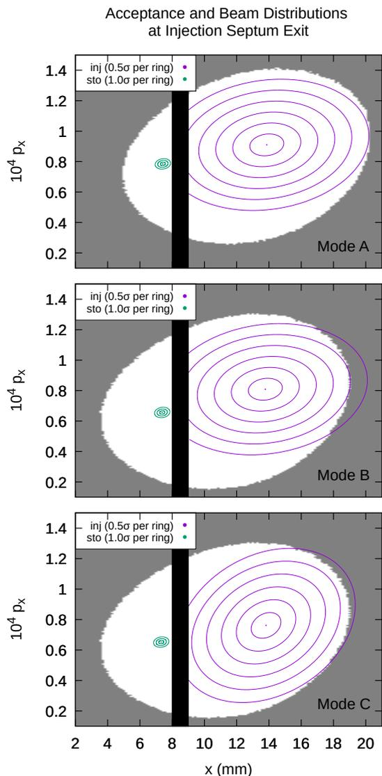
350 FIG. 5. Injected and stored beam profiles out to  $3\sigma$  at septum
