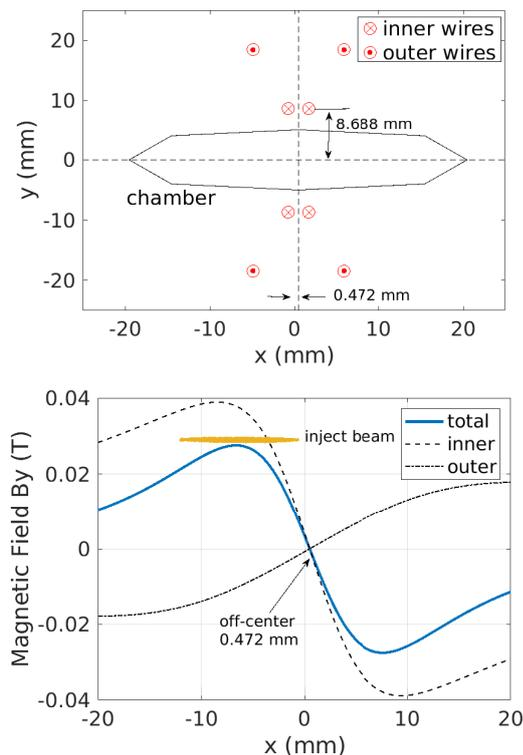
FIG. 15. NLK-design concept. Top: main conductors’ transverse positions (the return conductors are not shown). Bottom: magnetic-field profile in the mid plane.
