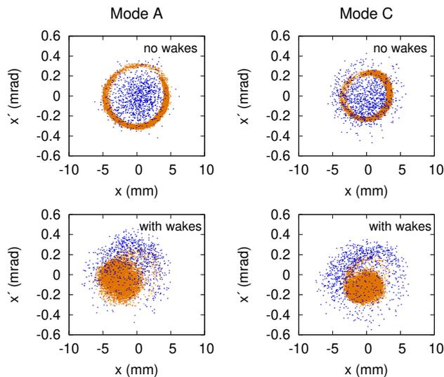
FIG. 11. Horizontal phase space of the stored (orange) and injected (blue) bunches after 2000 turns, without wakes (above) and with nominal wakes (below). The left figures show the results for Mode A, the right for Mode C.
