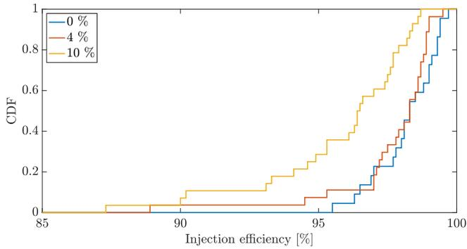
FIG. 9. Sensitivity of the injection efficiency to the non-uniformity of the injection kickers' pulse profile. The three data sets correspond to a 0%, 4%, and 10% sloping of the pulse profile. The simulation is conducted with a complete set of errors including shot-to-shot variation of the kick and septa strengths, as well as septum leakage fields.
