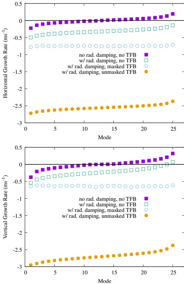
FIG. 14. Per-mode growth rates of a 25 bunch train in the accumulator ring determined by multi-bunch macro-particle tracking with resistive wall wake fields. During steady-state, all RW modes are safely damped with a total growth rate of about  $-2.5 \text{ ms}^{-1}$ . During the injection transient the effectiveness of the TFB is significantly diminished by the necessity of masking the 4 buckets into which charge is injected, though all modes remain damped.
