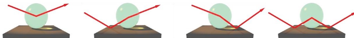
Figure 1.19: The four distinct possibilities involving reflection and refraction of the incident beam addressed using the Distorted-Born Wave Approximation. Reproduced from reference 29.
