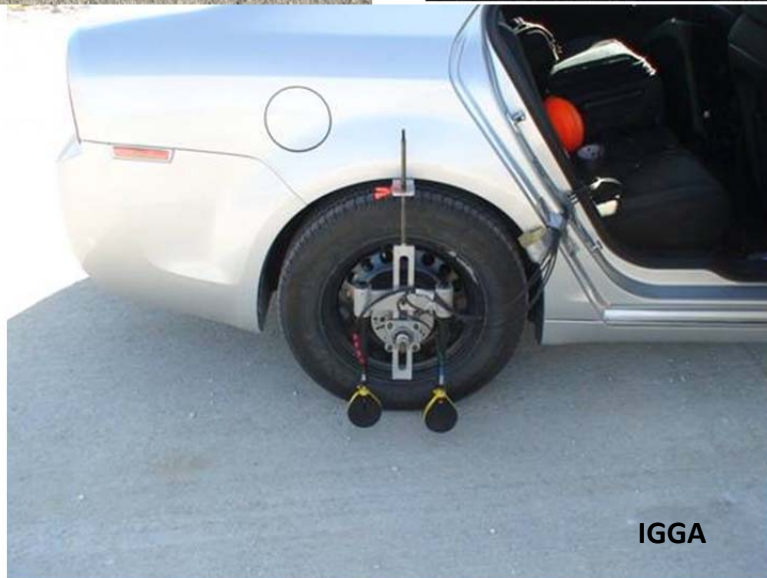
Figure 3: OBSI fixtures on IR, UC PRC, and IGGA test vehicle
