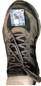
Figure 5.3: Indoor localization with a signal foot mounted inertial sensor.
