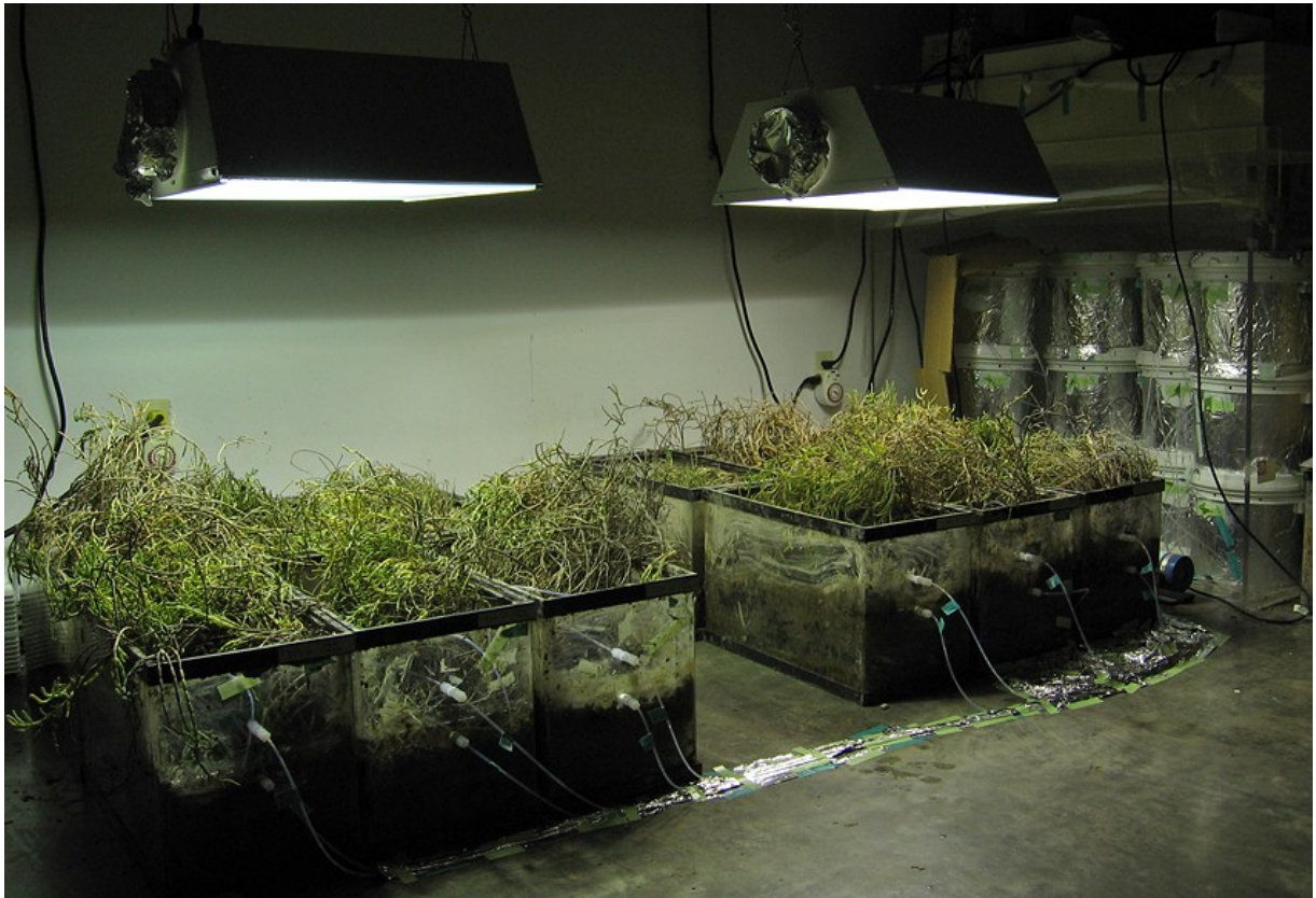
Figure 2-1. Laboratory microcosm setup used for the two experiments. The vegetated microcosms are shown, and this image was taken during the initial setup before the aluminum foil was added to the sides of the tanks up to the height of the sediment surface.
