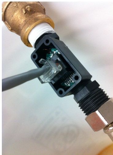
Figure 3.1.2 Fabricated, assembled flow meter
