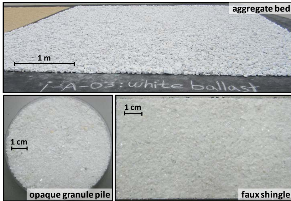
Figure 4.7.1: Aggregate bed, opaque granule pile, and shingle prepared from white ballast
