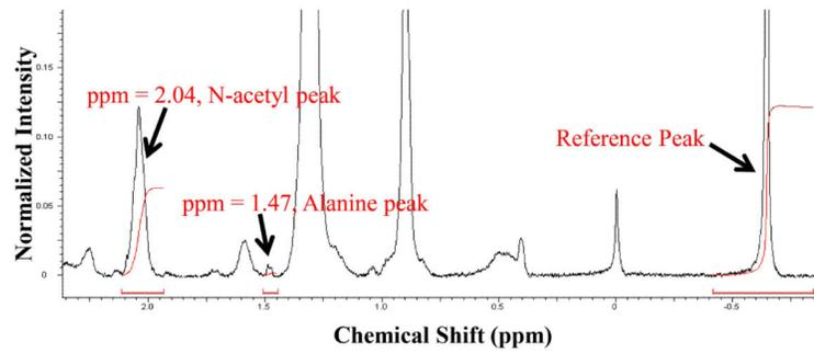
**Figure 2.** Example of HRMAS NMR spectrum acquired from a pair of OA cartilage plugs. Spectral data was referenced to TSP at 0 ppm. Peaks quantified include the N-acetyl singlet at ppm = 2.04 and, when present, the Alanine doublet at ppm = 1.47. The red curves under each quantified peak were generated by the program to depict their integration visually.
