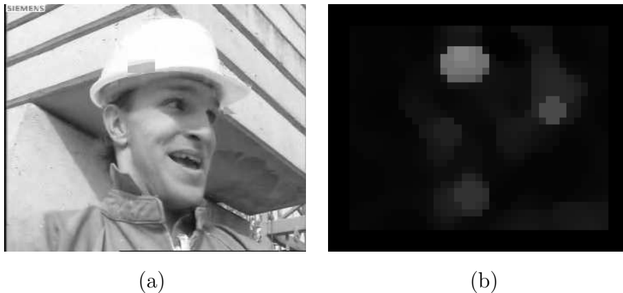
Figure 6.6: An example of DSM determination, where (a) a noticeable local distortion appears around the edge of the helmet, and (b) the corresponding DSM indicates a high value on those regions.
