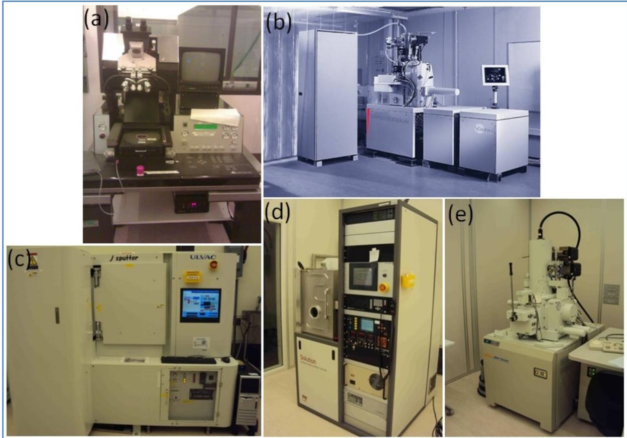
Figure 6.9: Images of nanofabrication equipments used for (a) photolithography (b) e-beam lithography, image obtained from <http://www.vistec-semi.com> (c) NiFe sputter deposition (d) Ni e-beam evaporation (e) scanning electron microscopy
