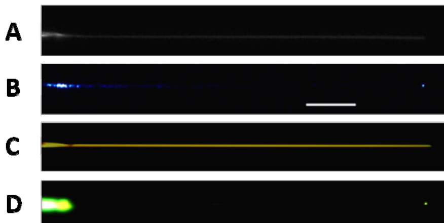
Figure 4.7 Fabrication of pH sensitive nanoprobe. A , dark field image of a probe before the coating of fluorescent polymer. B , waveguiding of 442nm laser coupled into the probe. C , Dark field image of a probe after polymer coating. D , PL image of the dye-coated probe in air. Scale bar: 5 \mu\text{m}
