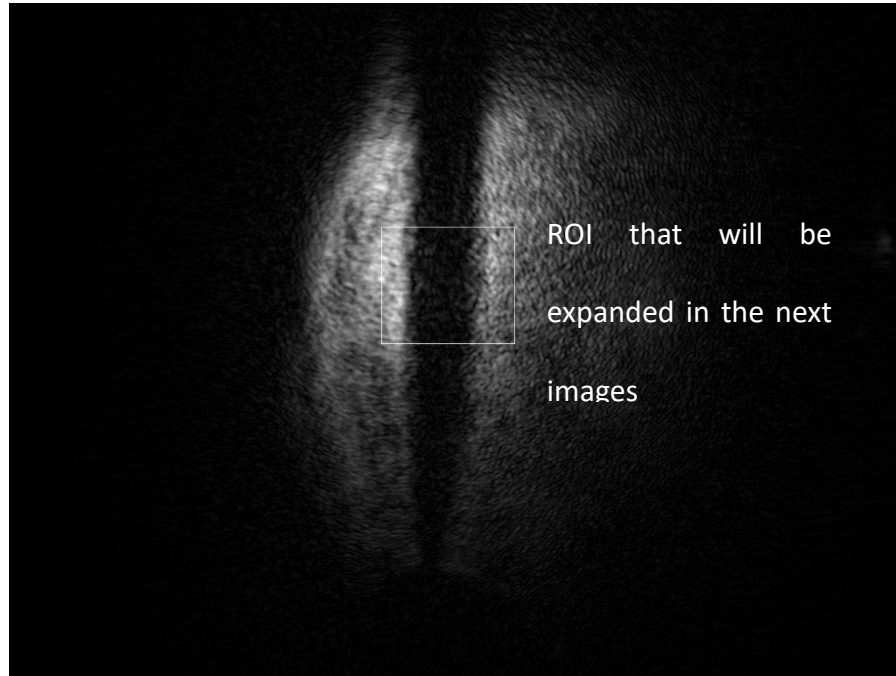
Figure 7.16 Dodecane spray injected at 1800 bar, chamber at ambient temperature and pressure.
