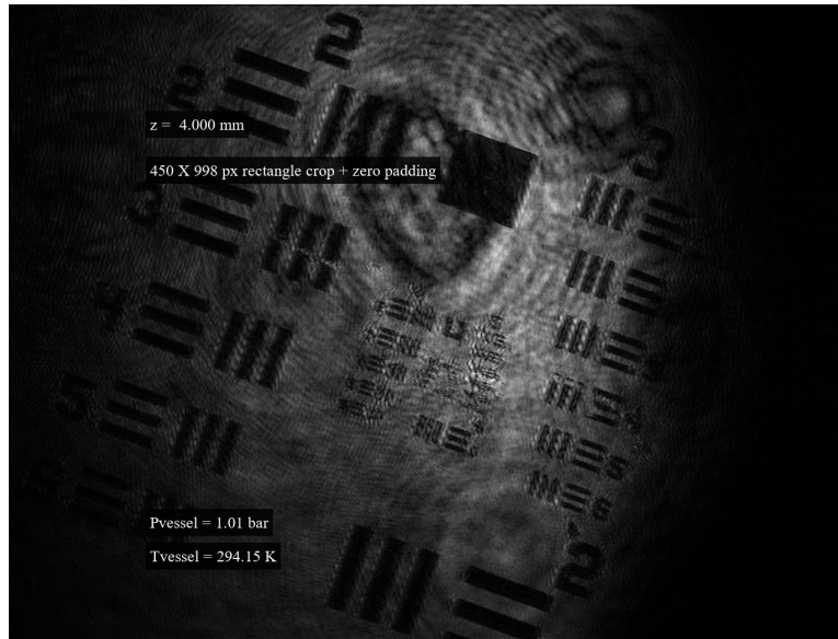
Figure 10.18 Reconstructed off-axis hologram of a USAF resolution chart placed at the center of the pressure vessel at the fuel injector location, z=4\text{mm} , 450 \times 998\text{px} reconstruction mask, d_o=35\text{ cm} d_i=40 M=1.14 f=180\text{mm}
