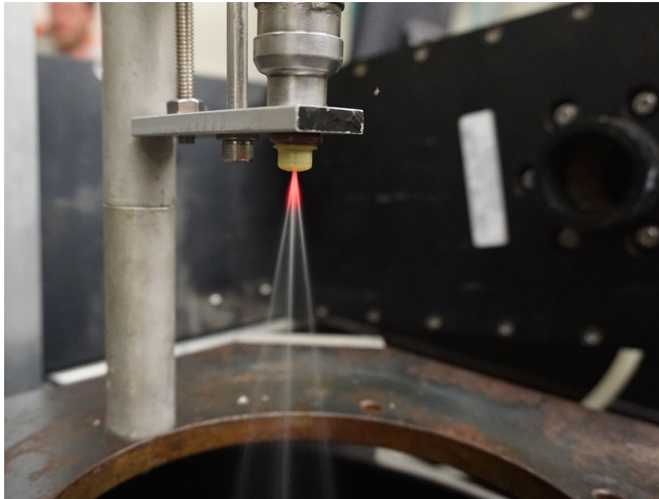
Figure 6.7 Laser diffraction particle sizing of the near nozzle region of the fuel injector. Water injected at approximately 80 PSI.
